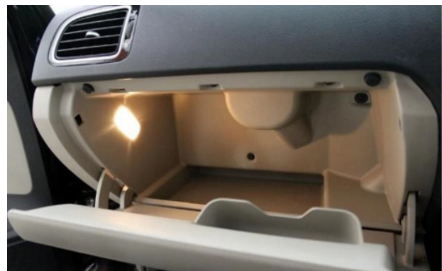
Figure 13: Glove box lamp application
