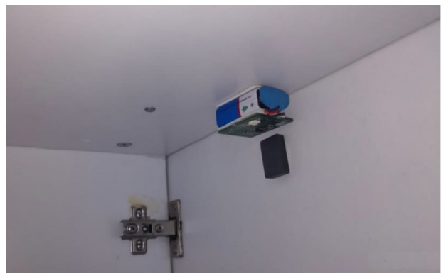
Figure 11: Inner cabinet lighting (LED turns off when door closes)
