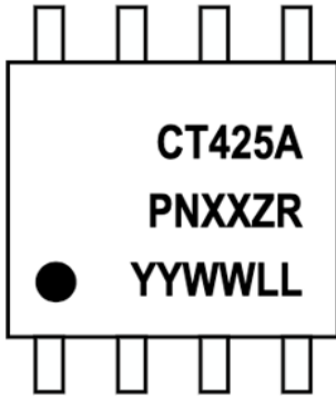
Figure 22: CT425 Device Marking for 8-lead Package
