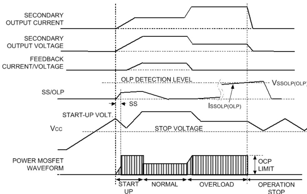
**Figure 9 – Timing at overload**
