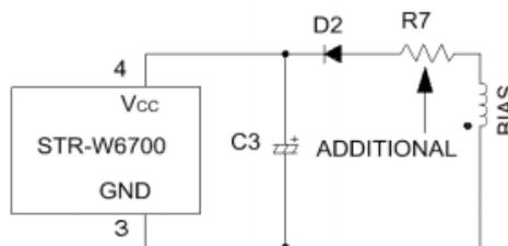
Figure 5 –  $V_{CC}$  peripheral circuit with R7
