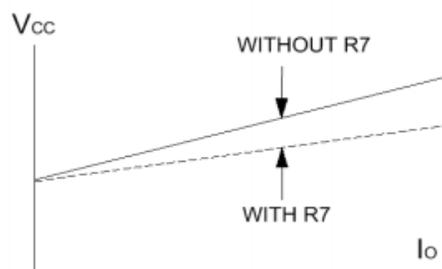
Figure 4 –  $V_{CC}$  vs.  $I_O$  (secondary load)
