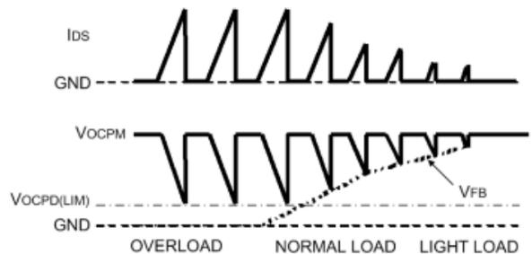
Figure 12 – Constant-voltage control (quasi-resonant signal ruled out)
