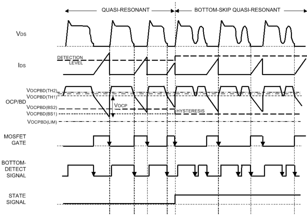
Figure 16 – Quasi-resonant to bottom-skip operation timing
