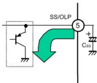
Figure 10 – Reset circuit at power turn OFF
