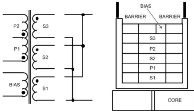
Figure 22 – Example of low-output voltage transformer
