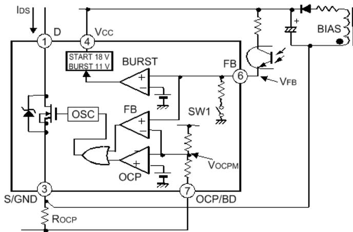
Figure 13 – REG functional block diagram
