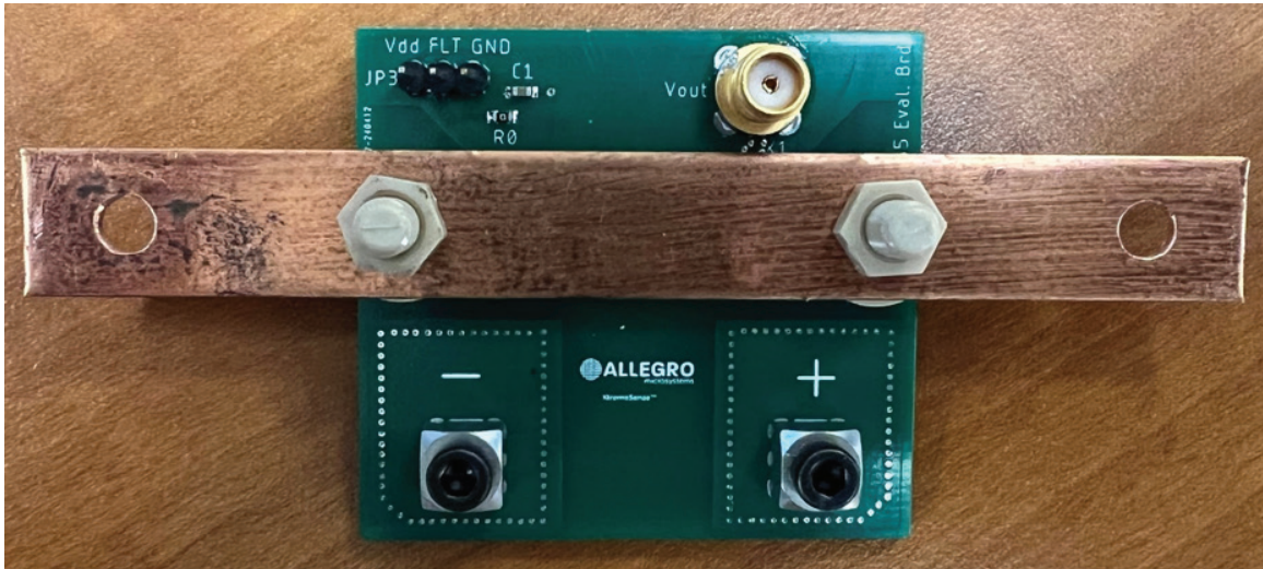
Figure 2: Evaluation Board with Busbar
