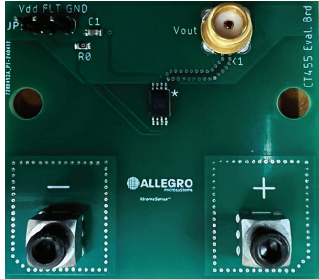
Figure 1: CT455 Evaluation Board (CTD455)
