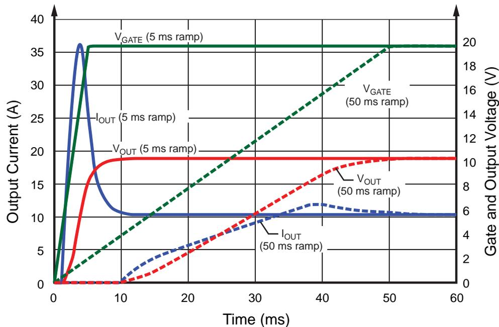
Figure 3. Hot-swapping current-surge suppression simulation
