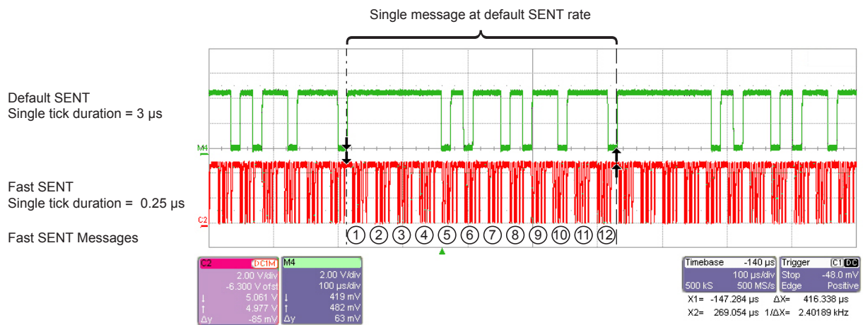
Figure 19. Comparison of time required to output (top) a default SENT mode message, and (bottom) a Fast SENT mode message
