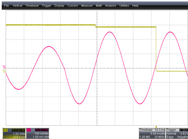
Figure 6. Overvoltage VRMS detection after 3 Half Cycle
