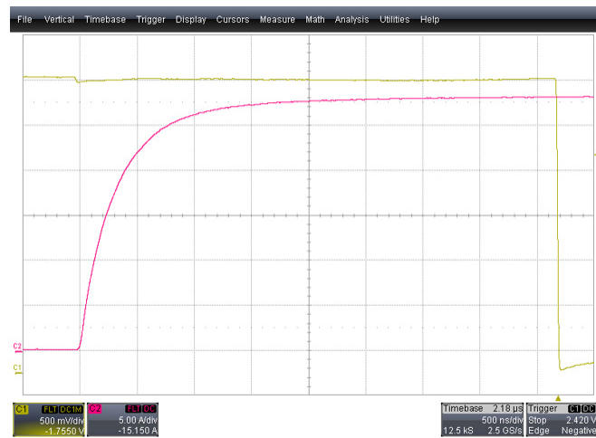
Figure 9. DIO_1 Overcurrent Fault Response with ftdly 0
