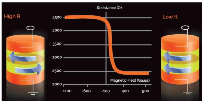
Figure 2: TMR Physical Principle for Single MTJ—MTJ Resistance Depends on Magnitude of External Magnetic Field
