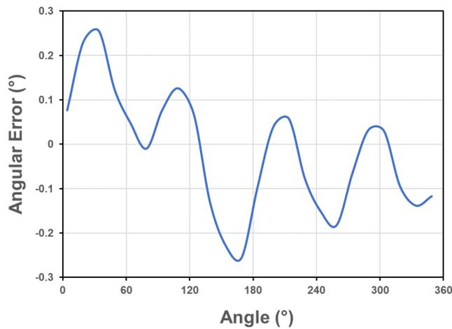
Figure 6: Example of Angle Error (AE) as a Function of Magnetic-field angle Measured at Room Temperature at a Single Magnitude Rotating Magnetic Field
