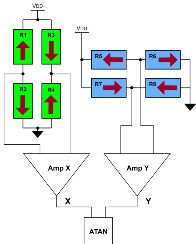
Figure 5: X and Y Bridges of TMR Angle Sensor, Together with Readout Circuit Block Diagram and Arctangent Calculation Block
