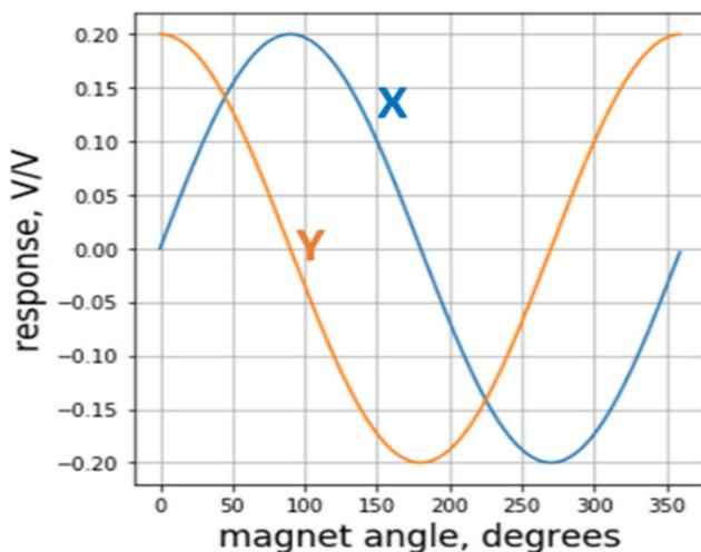
Figure 4: X and Y Bridge Response as Function of External Magnetic-field angle
