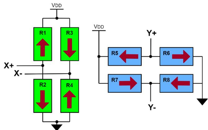
R1, R2, R3, R4 Wheatstone bridge is sensitive to north/south orientation of magnetic field (X). R5, R6, R7, R8 Wheatstone bridge is sensitive to east/west orientation of magnetic field (Y).
