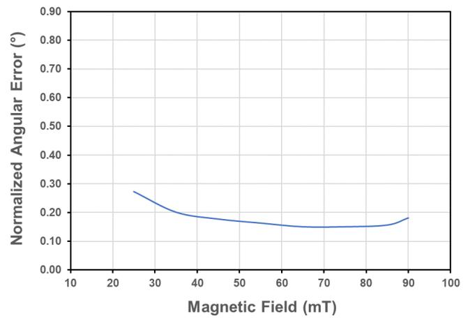
Figure 7: Example of Normalized Angle Error versus Magnitude of a Rotating Magnetic Field Measured at Room Temperature
