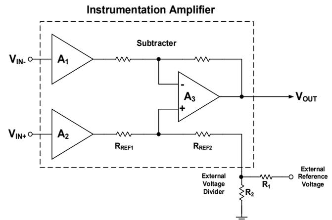
Figure 8: Conversion of Differential Analog Signal into Single-Ended Signal with Reference Voltage Shift on the INA
