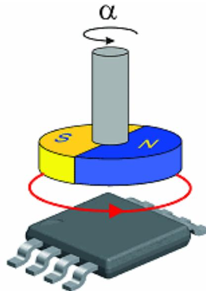
Figure 1: Angle Sensor Measures Magnetic-field angle of Shaft End
