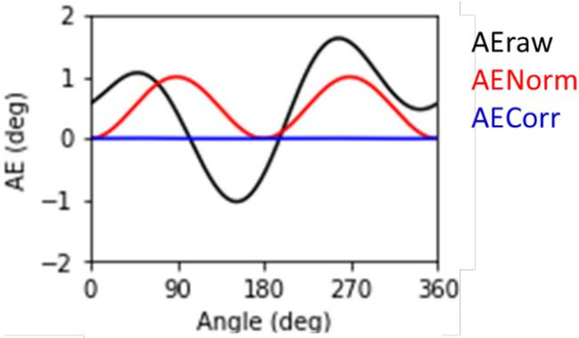
Figure 8: Angular dependence of AE for 2D sensor with  $\text{Sync} = 1.02$ ,  $C_{SIN} / A_{SIN} = 1\%$  and  $\alpha_{COS} = 1.0^\circ$ . AErAw (black curve) refers to the AE derived without any correction method. AENorm (red curve) refers to the AE derived from normalization correction. AECorr (blue curve) refers to the AE derived from nonorthogonality correction method.
