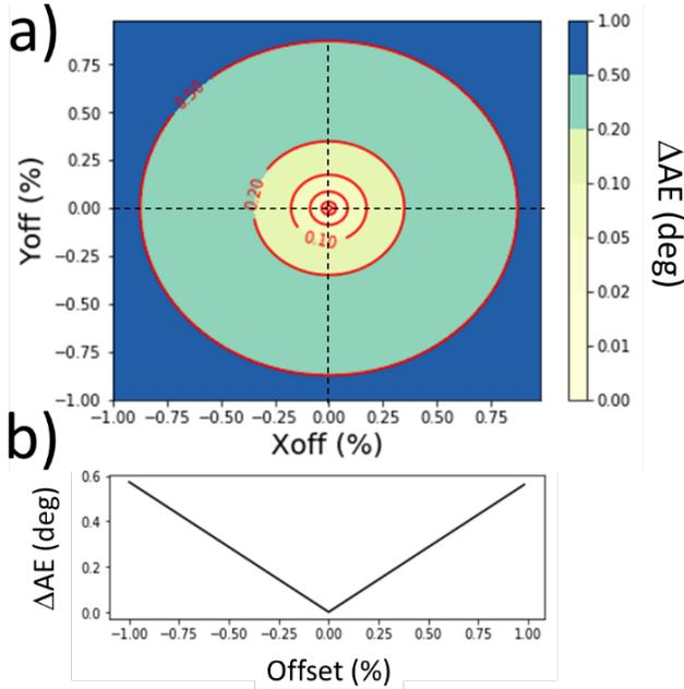
Figure 5: a) Increase of AE due to offset increase on both bridges, where  $\Delta X_{off}$  and  $\Delta Y_{off}$  are the variation ratio of both offset voltages; b)  $\Delta AE$  vs.  $\Delta Total$  Offset.
