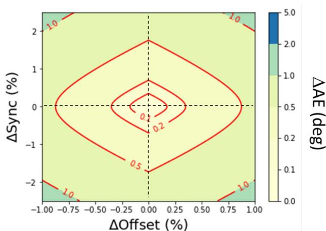
Figure 10:  $\Delta AE$  map vs.  $\Delta Sync$  and  $\Delta Offset$ . Here, nonorthogonality was considered ( $\alpha_{COS}$  and  $\alpha_{COS} = 0$ ).
