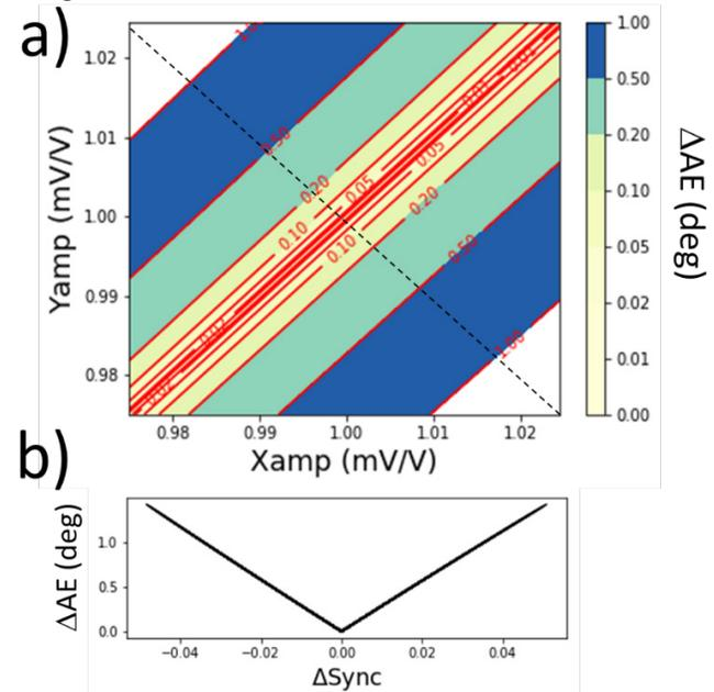
Figure 4: a) Increase of AE due to amplitude increase on both bridges, where  $\Delta X_{amp}$  and  $\Delta Y_{amp}$  are the variation ratio of both amplitude voltages., and the dashed lines show increase of Sync direction; b)  $\Delta AE$  vs.  $\Delta Sync$ .
