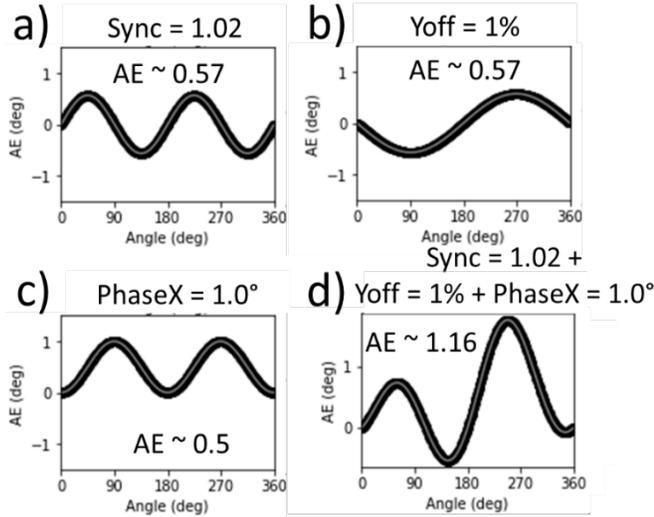
Figure 7: Angular dependence of AE for a)  $Sync = 1.02$ ,  $C_{COS} = C_{SIN} = 0$ , and  $\alpha_{COS} = \alpha_{SIN} = 0$ ; b)  $Sync = 1.0$ ,  $C_{SIN}/A_{SIN} = 1\%$ ,  $C_{COS} = 0$ , and  $\alpha_{COS} = \alpha_{SIN} = 0$ ; c)  $Sync = 1.0$ ,  $C_{COS} = C_{SIN} = 0$ ,  $\alpha_{SIN} = 0$ , and  $\alpha_{COS} = 1.0^\circ$
