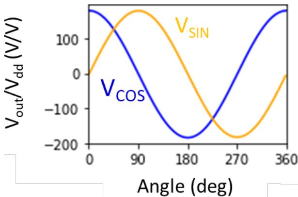
Figure 3: Typical angular dependence of the output voltage of a 2D magnetic sensor with two Wheatstone bridges, one orthogonally oriented with respect to the other.
