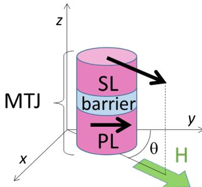
Figure 1: Effect of External Magnetic Field,  $H$ , on MTJ Cell
