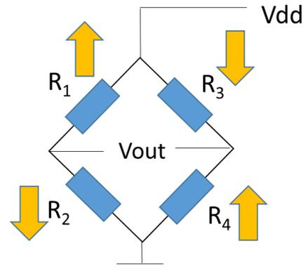
Figure 2: Schematic of a Wheatstone bridge architecture with 4 MTJ branches. Arrows show the orientation of the PL for each MTJ branch.
