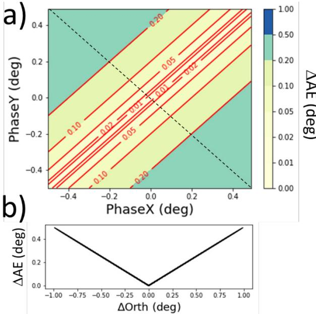
Figure 6: a) Increase of AE due to phase-shift increase on both bridges, where the dashed lines show increase of nonorthogonality; b)  $\Delta AE$  vs.  $\Delta Orth$ .
