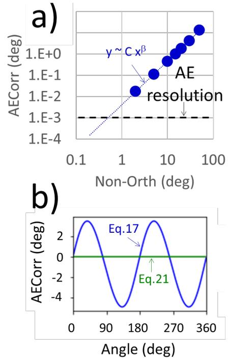
Figure 9: a) AECorr (determined by Equation 20) vs. nonorthogonality. Black dashed lines indicate the usual AE resolution in a 2D magnetic sensor.  $C \sim 0.0041$  and  $\beta \sim 2.04$ ; b) angular dependence of AECorr with nonorthogonality of  $30^\circ$  when determining AECorr by Equation 20 (blue curve) or by Equation 24 (green curve).
