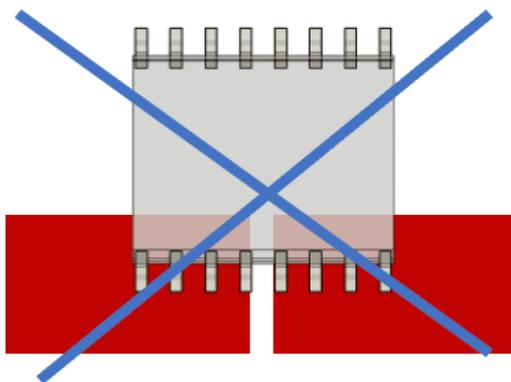
Figure 1: Overview of CT43x in SOICW-16 Package on a PCB with a Current Trace
