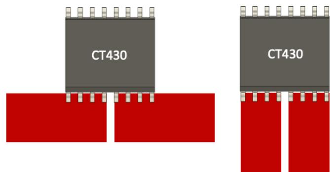
Figure 19: Recommended Layouts of Current-Carrying Trace
