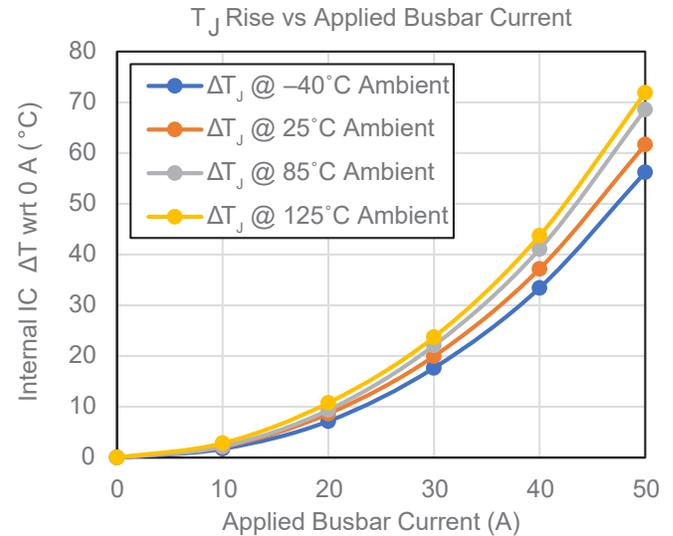
Figure 15: Junction Temperature of CT43x vs. Applied Current through Busbar
