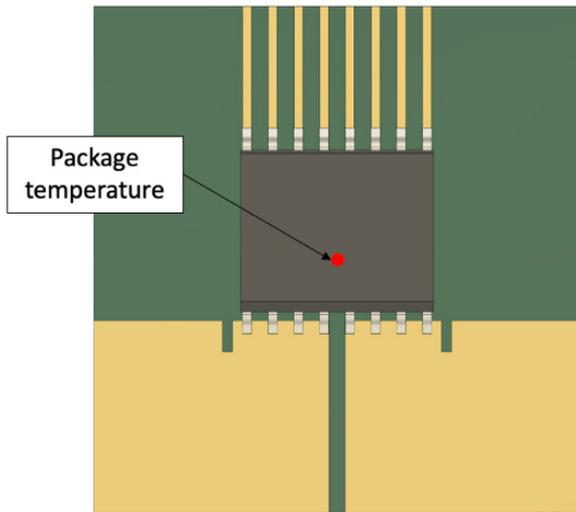
Figure 14: CT43x SOICW-16 with Red Dot Showing Relative Hottest Point on Package
