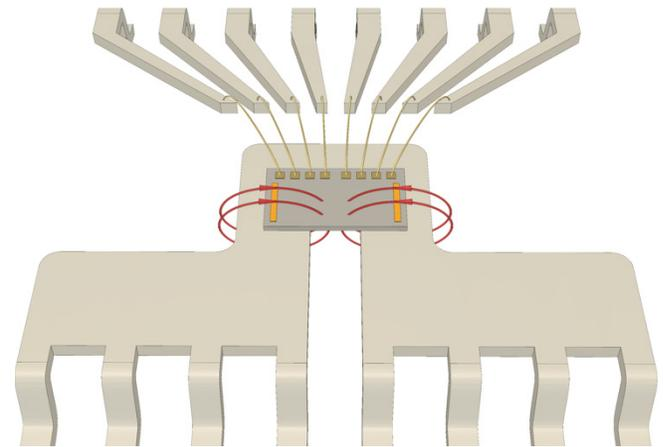
Figure 18: CT43x Leadframe Approximation Showing Internal U-Shape that Allows Differential Sensing Capability
