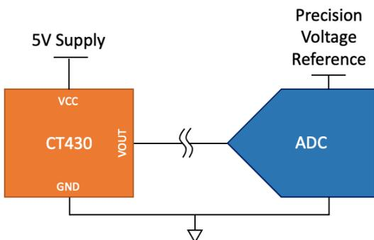
Figure 4: CT43x Connected to Single-Ended ADC
