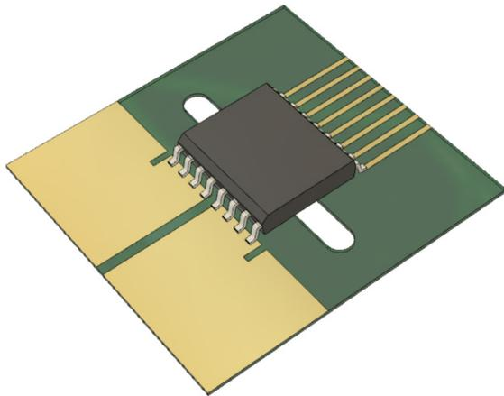
Figure 12: CT43x PCB with Slit to Increase Creepage
