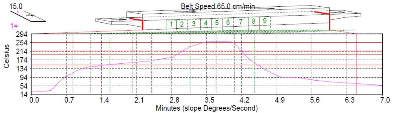
Figure 20: Lead-Free Solder Temperature Profile and Belt Speed for Allegro TMR Products
