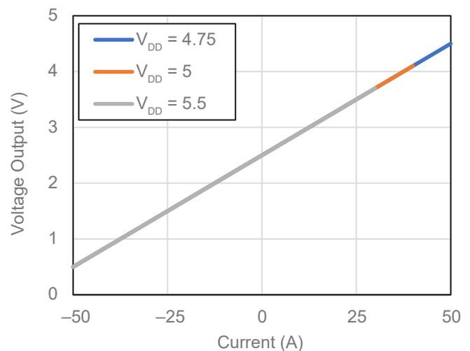
Figure 2: CT43x Output Voltage Gain and Offset Do Not Vary with a Varying Voltage Supply on the VCC Pin
