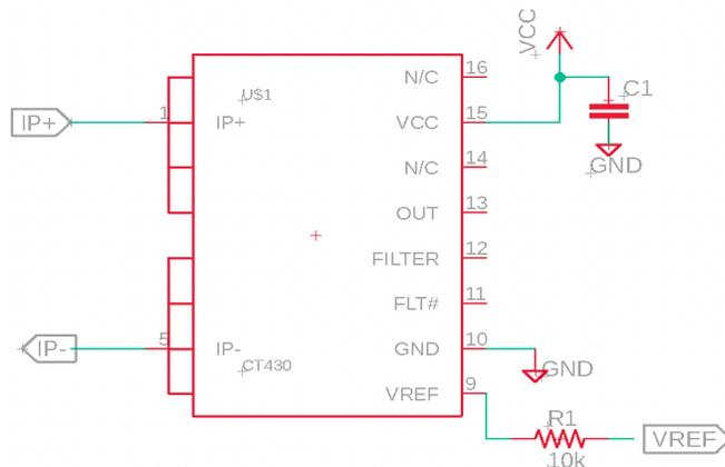
Figure 6: CT43x with 10  $\text{k}\Omega$  R1 Resistor Connected in Series to VREF Pin
