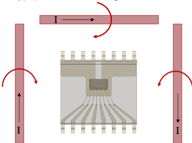
Figure 17: CT43x with Three Adjacent Current-Carrying Conductors (shown in red)
