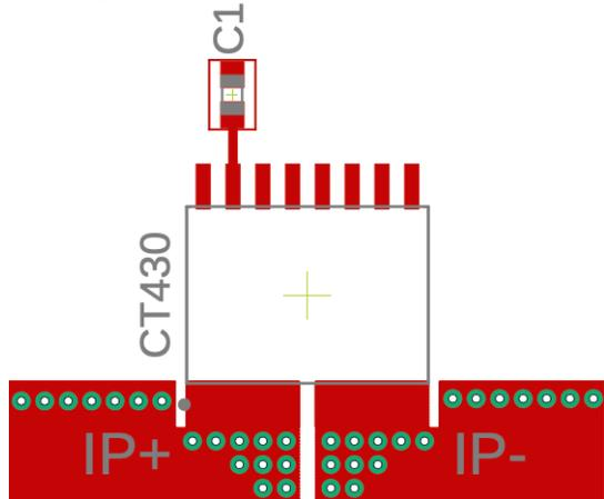
Figure 3: CT43x Footprint with Decoupling Capacitor C1
