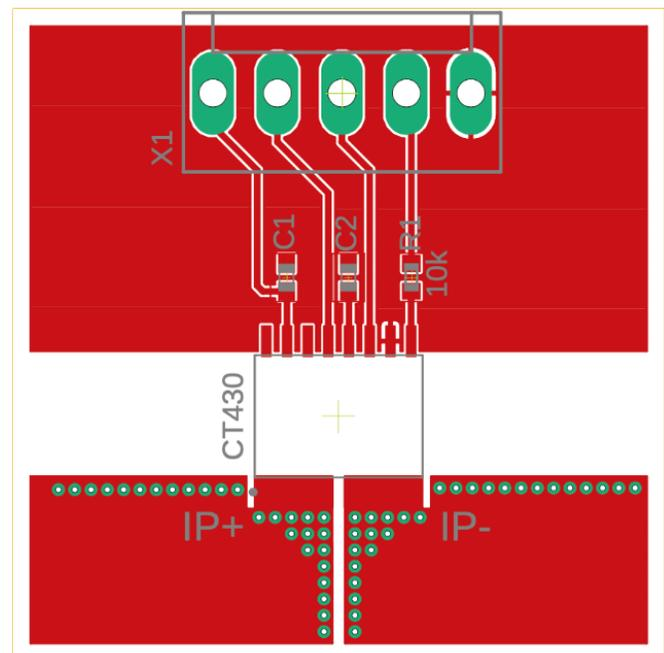
Figure 8: Layout of Current-Carrying Trace and Signal Traces
