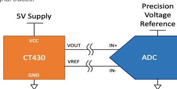
Figure 5: CT43x Connected to Differential ADC Input
