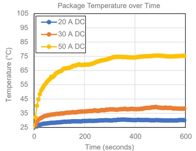
Figure 16: Package Temperature of CT43x over Time
