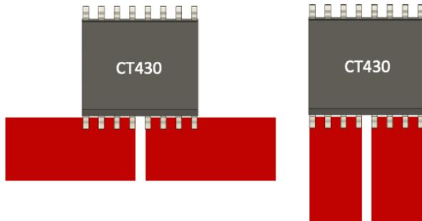
Figure 9: Recommended Layouts of Current-Carrying Trace
