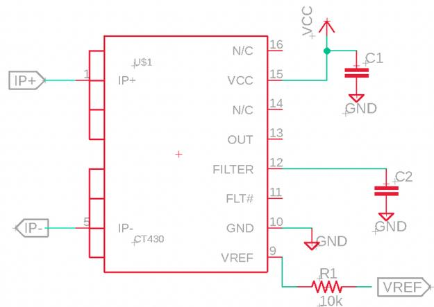
Figure 13: CT43x Using Capacitor C2 to Implement Low-Pass Filter
