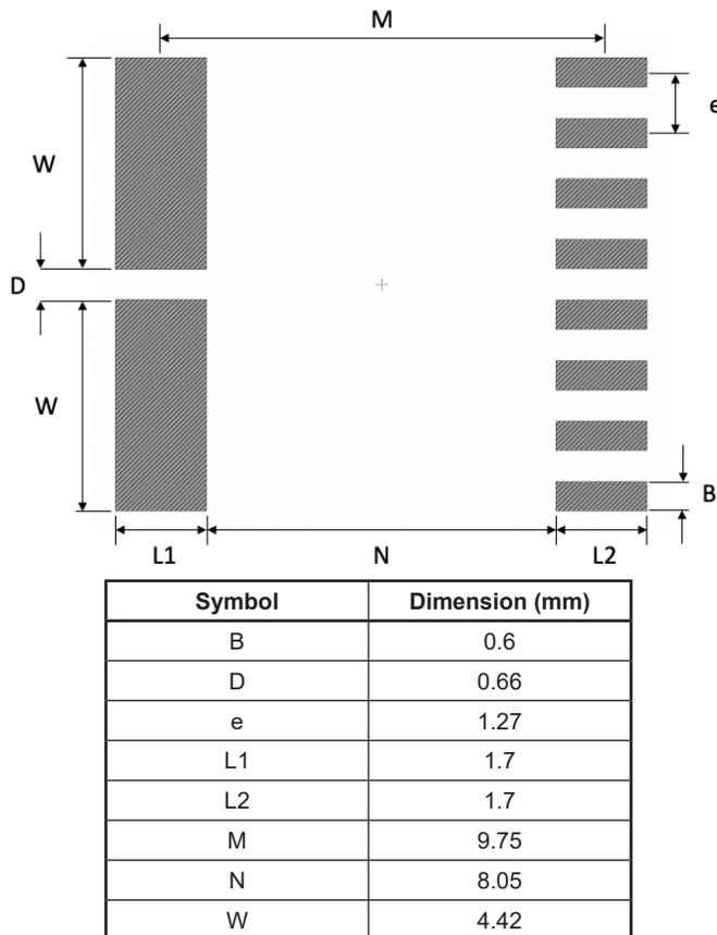
Figure 7: CT43x SOICW-16 Recommended Footprint
