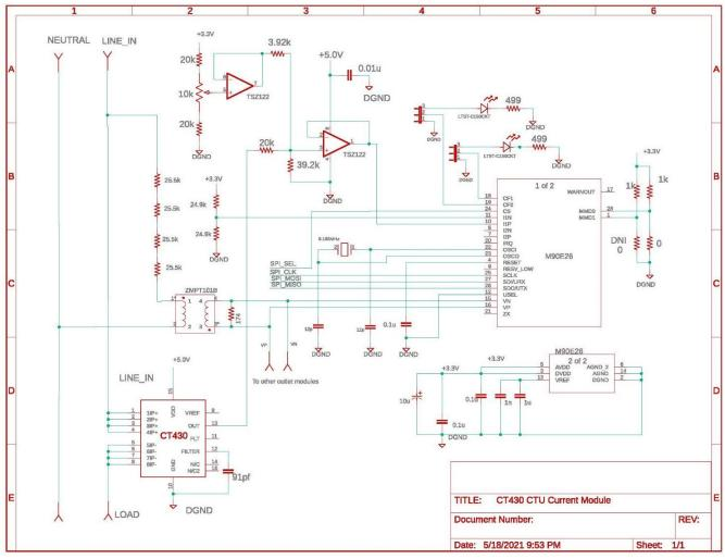
Figure 6: CT430 PDU Outlet Module
