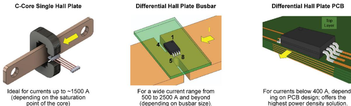
Figure 1: Examples of a busbar with a C-core (left), notched busbar with a coreless differential Hall sensor (middle), and coreless PCB design (right)
