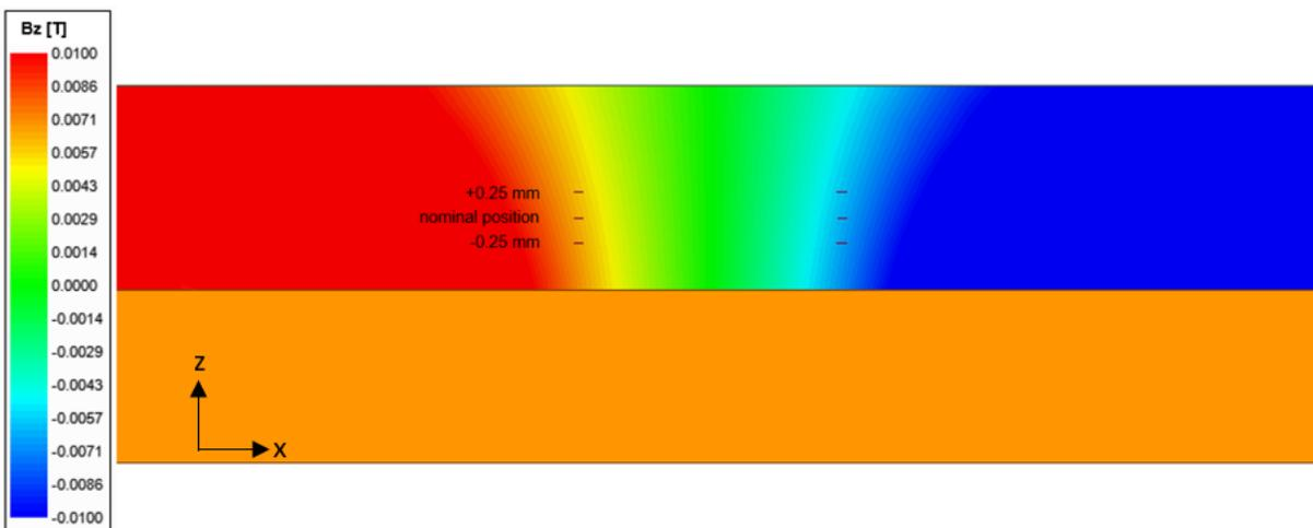
Figure 2: B<sub>z</sub>-Field for a notch width of 8 mm. The scale is cut to ±0.01 T to show the B<sub>z</sub> gradient at the Hall plate locations.
