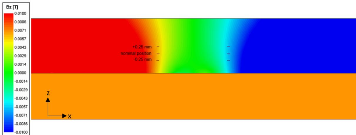
Figure 3: Bz-Field of a DC Q-Rift PCB. Bz-Field for a notch width of 8 mm. The scale is cut to  $\pm 0.01$  T to show the Bz gradient at the Hall plate locations.
