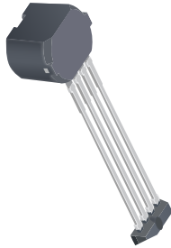
Figure 1: Sensor IC package used in the simulation.
