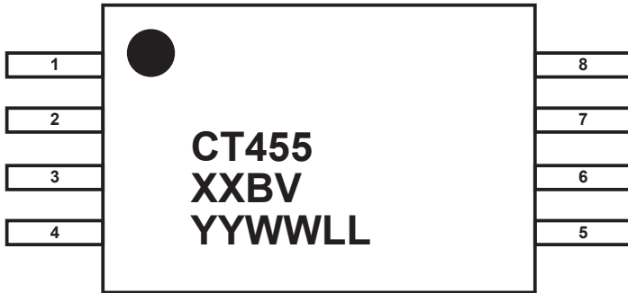
Figure 23: CT455 Device Marking for Eight-Lead TSSOP Package
