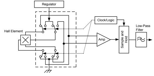
**Concept of Chopper Stabilization Technique**
