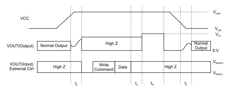
Figure 15: Write to Non-Volatile Memory (EEPROM)
