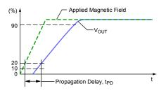
**Figure 3: Propagation Delay Definition**
