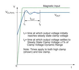
Figure 2: Delay to Clamp Definition
