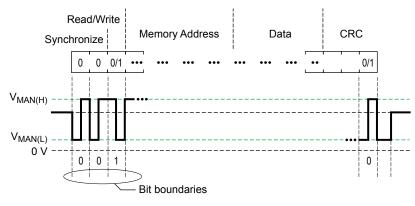
Figure 10: General Format for Serial Interface Commands
