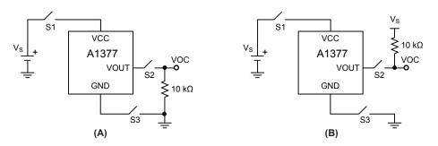
Figure 9: Diagnostic Application Circuits: (A) Pull-Down, (B) Pull-Up
