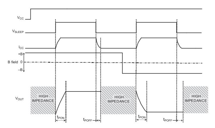
Figure 1. A139x Timing Diagram
