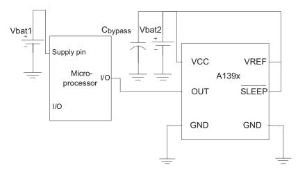
Figure 2. Application circuit showing sleep mode disabled and output ratiometric to the A139x supply.
