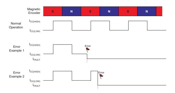
Figure 6: Output Protocol with ASIL Safety Current
