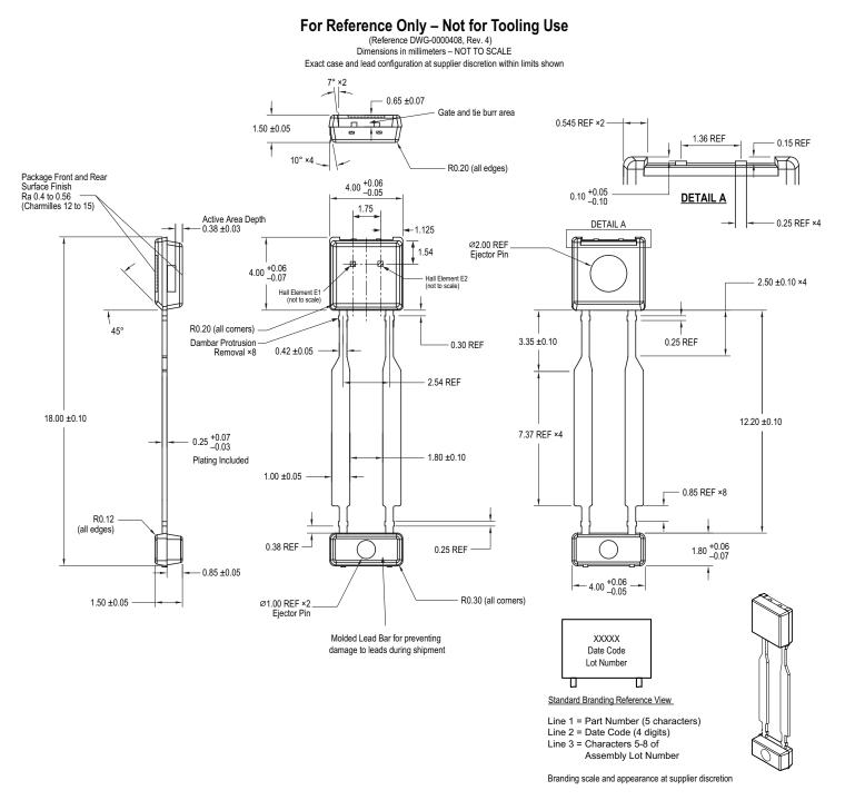
Figure 7: Package UB, 2-Pin SIP
