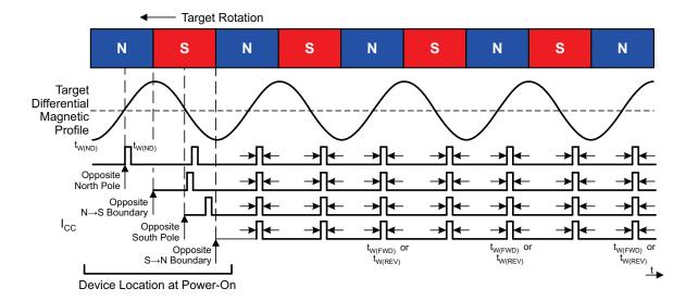
Figure 12: Calibration Behavior of the -xPx Variant
