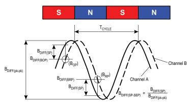
Figure 5: Definition of Switch Point Separation
