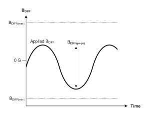
**Figure 6: Input Signal Definition**
