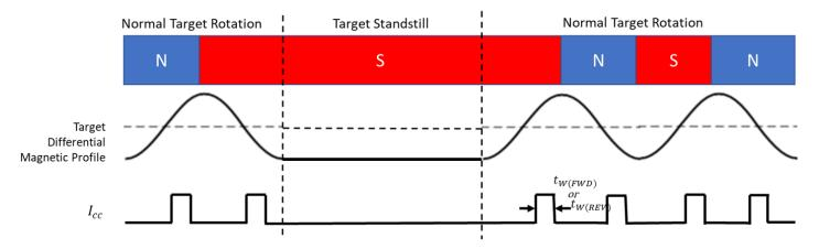
Figure 14: Standstill, -xxM Variant
