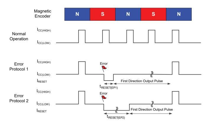
Figure 11: Output Protocol of the -xBx Variant (ASIL Safe State)
