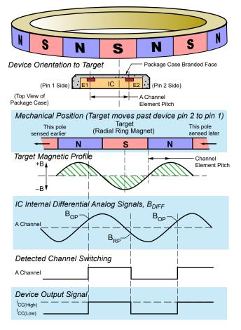
Figure 6: Basic Operation (Ring Magnet)
