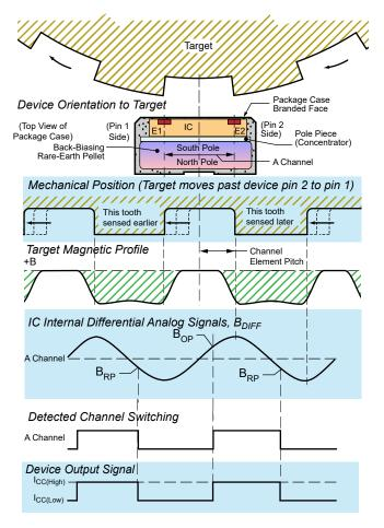
Figure 8: Basic Operation (Back-Biased Solution)
