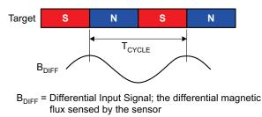
T<sub>CYCLE</sub> = Target Cycle; the amount of rotation that moves one north pole and one south pole across the sensor
