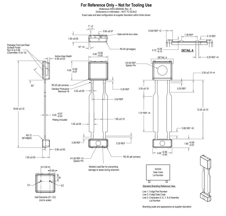
Figure 10: Package UB, 2-Pin SIP
