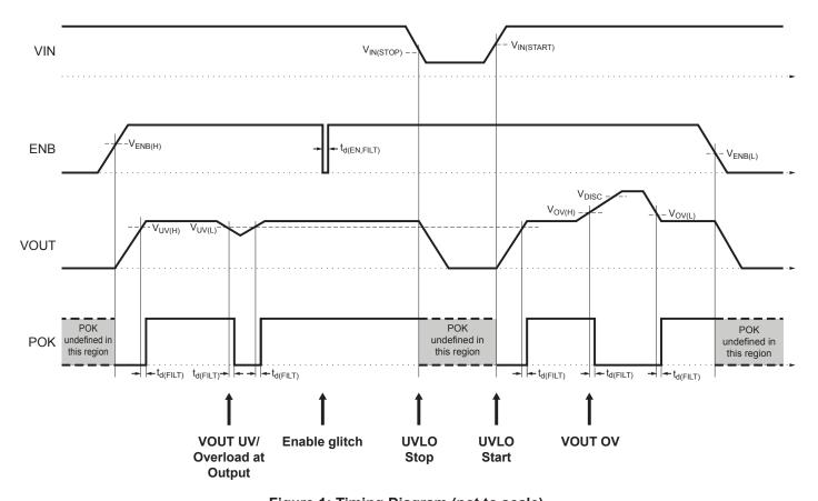
Figure 1: Timing Diagram (not to scale)
