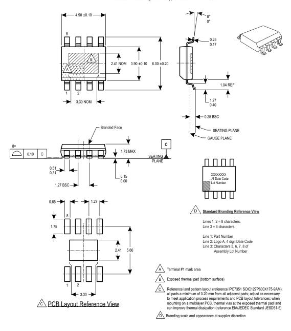
Figure 5: Package LJ, 8-Pin eSOIC
