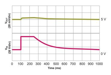
**Load Transient Response** ( $V_{IN}$  = 12 V,  $I_{OUT}$  = 5 mA to 50 mA,  $C_{OUT}$  = 4.7  $\mu$ F)
