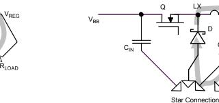
Figure 6. FET off-cycle current conduction paths
