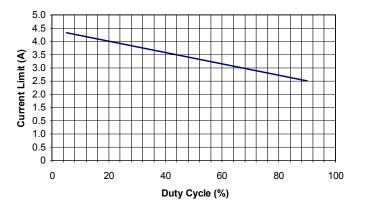
Figure 3. Current limit versus duty cycle
