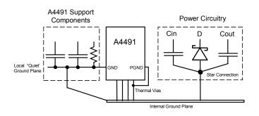
Figure 4. Ground plane configurations
