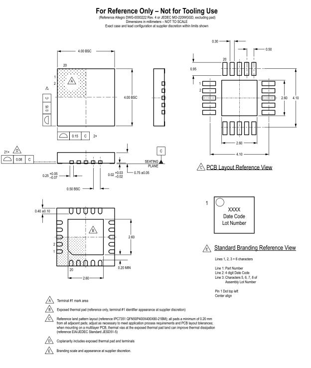
Figure 9: Package ES, 20-Pin QFN with Exposed Thermal Pad
