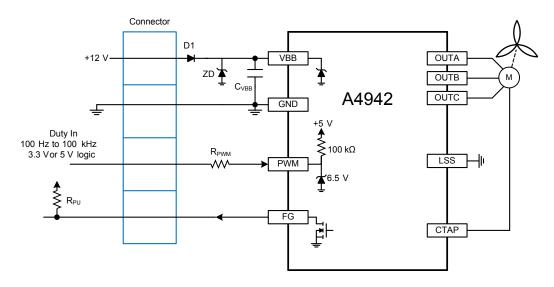
Figure 7: Typical Fan System Configuration
