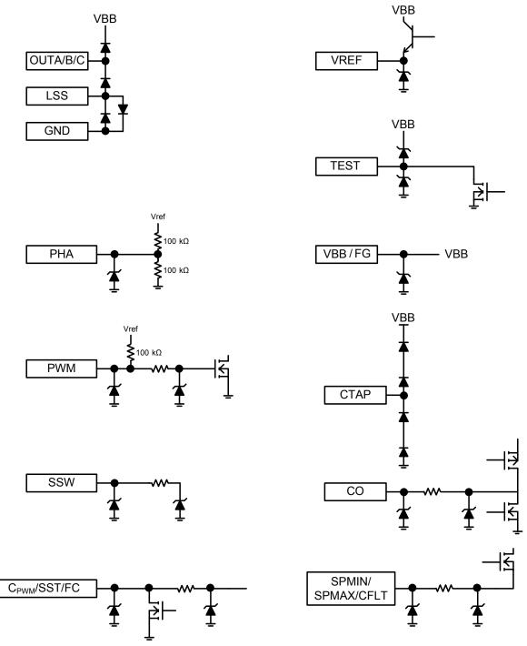
Figure 8: Pin Structures
