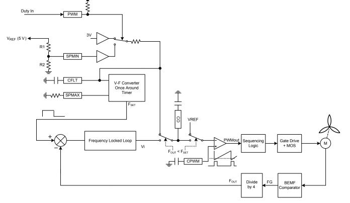
Figure 3: Equivalent Circuit of Closed Loop Control System
