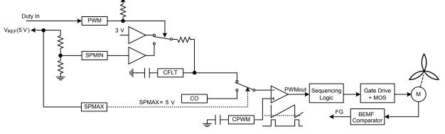
Figure 4: Equivalent Circuit of Open Loop Control System
