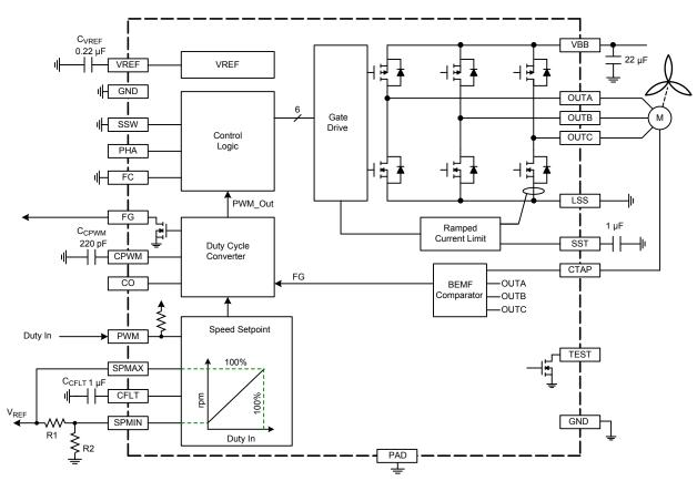
Figure 5: Functional Block Diagram Demonstrating Implementation of Open Loop Control
