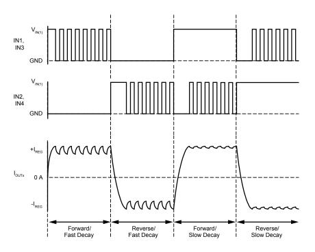
Figure 3: PWM Control Timing Diagram
