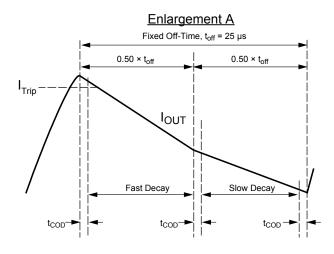
Figure 4: Mixed Decay Mode Operation
