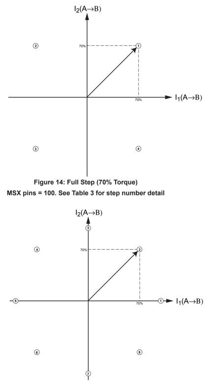
Figure 15: Half Step (70% Torque) MSX pins = 101. See Table 3 for step number detail
