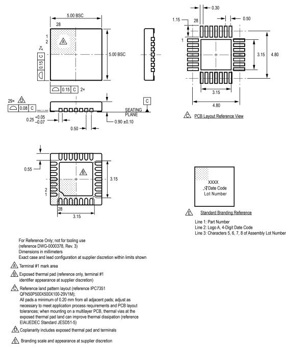
ET Package, 28-Pin QFN with Exposed Thermal Pad
