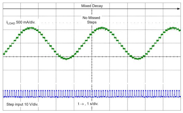
Figure 4: Continuous Stepping Using APFD (ROSC Pin Grounded)
