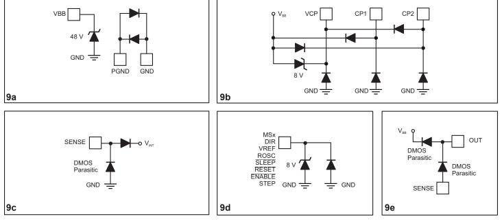
Figure 9: Pin Circuit Diagrams
