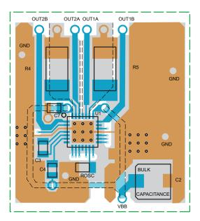
Figure 7: ET Package Circuit Layout
