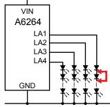
C. Current remains regulated. Matching may be affected. Only the shorted LED is inactive. FF is low
