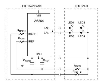
Figure 13. Application Circuit for Binning – Current-setting resistor ( $R_{\text{REF2}}$ ) can be placed on LED board for different bins of LEDs.
