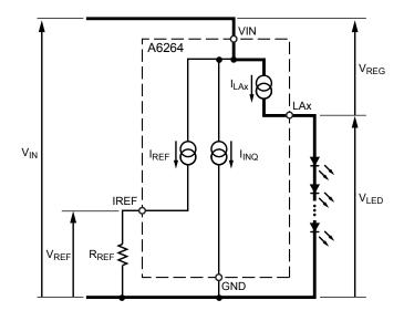
Figure 3. Internal power dissipation sources.
