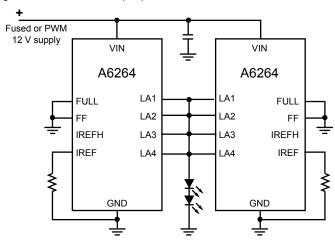
Figure 11. Disabling FF, driving high brightness (HB) LEDs with two A6264s.
