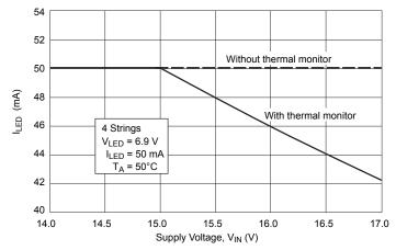
Figure 5. LED current versus Supply Voltage.
