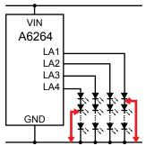
A. Any LED cathode short to ground. Current remains regulated in non-shorted LEDs. Matching may be affected. FF is low.
