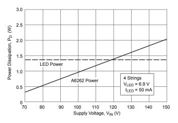
Figure 4. Power Dissipation versus Supply Voltage.
