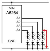
B. Any LAx output short to ground. Shorted output is disabled. Other outputs remain active. FF is high.
