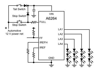
Figure 8. Common tail / stop lamp configuration.
