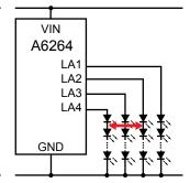
D. Short between LEDs in different strings. Current remains regulated. Current is summed and shared by affected strings. Intensity match dependent on voltage binning. FF is low.
