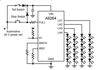
Figure 10. Higher voltage supply application.
