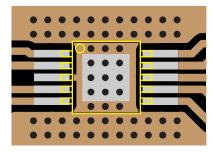
Figure 7. Board via layout for thermal dissipation: (top) LP package (bottom) LY package.
