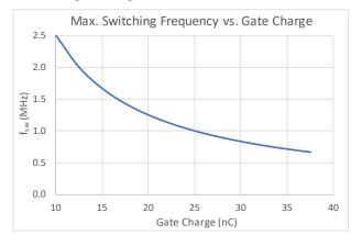
Figure 58: Maximum Switching Frequency vs. Gate Charge (to keep average  $V_{DRV}$  current under 25 mA).
