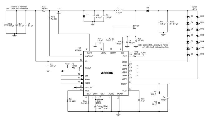
Figure 51: Boost Design Example Schematic (f<sub>SW</sub> = 2.15 MHz)
