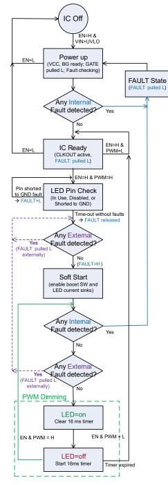
Figure 36: Simplified startup flow chart for A80606-1, showing responses to both Internal and External FAULT signals
