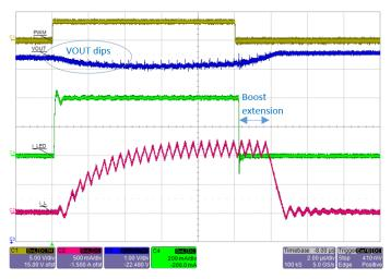
Figure 20: Traditional PWM Dimming operation where boost switch and LED current are enabled at the same time. Note that  $V_{OUT}$  shows overall ripple of ~0.5 V
