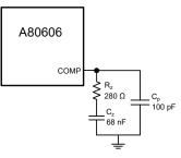
Figure 50: Compensation Network Schematic
