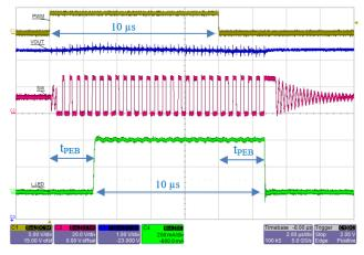
Figure 18: Zoom in view for PWM on-time = 10  $\mu$ s. Notice that the LED current is shifted with respect to PWM signal. Ripple at V<sub>OUT</sub> is ~0.2 V when using 2 × 4.7  $\mu$ F MLCC as output capacitors.
