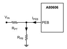
Figure 23: PEB delay setup circuit with connection to V<sub>IN</sub>
