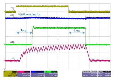
Figure 21: A80606 PWM dimming operation with PEB delay set to 3  $\mu s.$  Note that  $V_{OUT}$  ripple is reduced to ~0.2 V.
