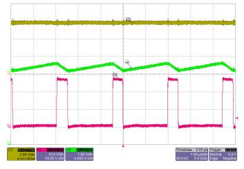
Figure 45: Normal 400 kHz switching waveform at  $V_{\rm IN}$  = 6 V. Red trace is the SW node voltage at 10 V/div. Green trace is the inductor current at 1 A/div.
