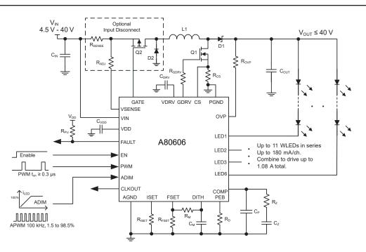
Figure 1: A80606 Simplified Circuit Configuration
