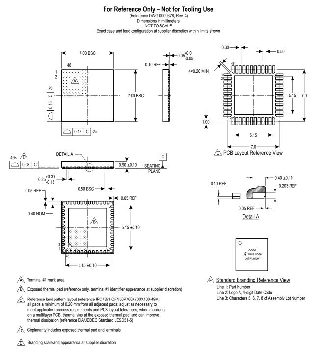
Figure 49: Package EV, 48-Pin 7 mm × 7 mm QFN with Exposed Thermal Pad and Wettable Flank
