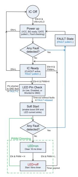
Figure 35: Simplified A80606 Startup Flowchart
