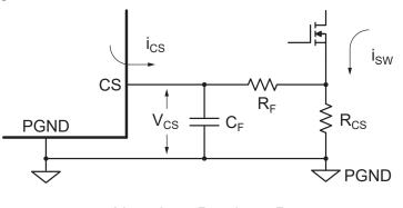
$$V_{CS} = I_{CS} \times R_F + I_{SW} \times R_{CS}$$
