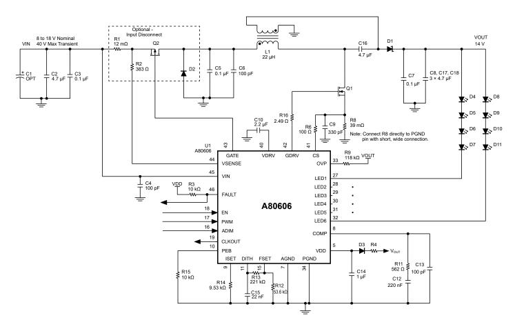
Figure 52: SEPIC configuration. Allows operation with  $V_{IN}$  both above and below  $V_{OUT}$ .
