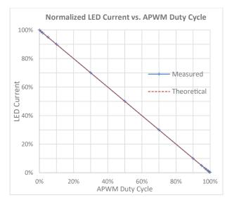
Figure 26: Showing LED current is inversely proportional to the APWM duty cycle. Test conditions:  $V_{IN} = 12 V$ ,  $V_{OUT} = 25 V$  (8 × WLED), total LED current = 100 mA × 4, APWM frequency = 100 kHz
