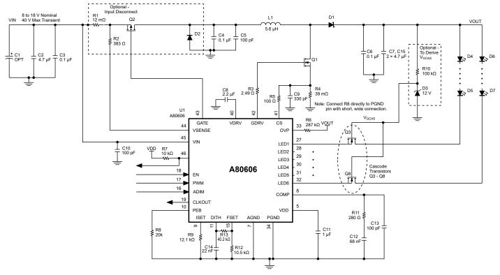
Figure 53: Cascode-Protected LED Pins Design.
