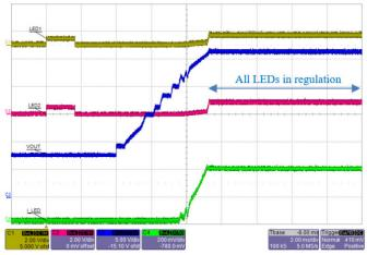
Figure 37: A80606 Normal startup sequence showing voltage at LED1 and LED2 pins.  $V_{IN}$  = 6 V, output = 8 × WLED in series, current = 4 × 100 mA
