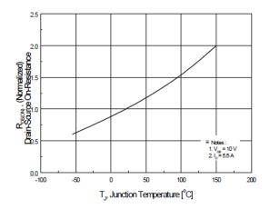
Figure 57: Nominalized On-Resistance vs. Junction Temperature at  $V_{GS}$  = 10 V. Note that resistance increases by 100% when temperature rises from 25°C to 150°C.
