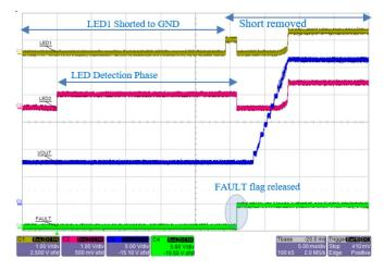
Figure 8: LED1 is shorted-to-GND initially, then released. After the fault is removed, the IC auto-recovers and proceeds with soft-start. FAULT is released at the end of LED detection phase.
