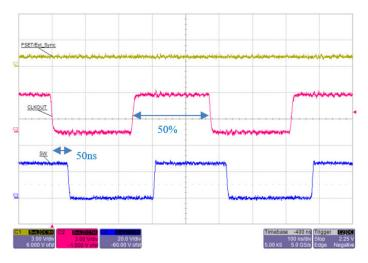
Figure 15: Without external sync, the CLKOUT signal has a fixed duty cycle of 50%. Delay from CLKOUT falling edge to SW falling edge is approximately 50 ns.
