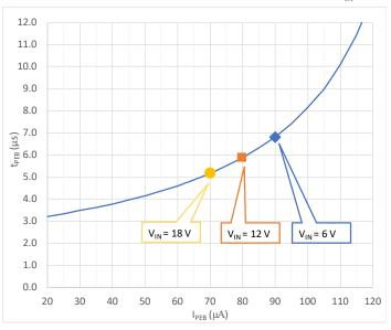
Figure 24: PEB delay t<sub>PEB</sub> vs. PEB pin current
