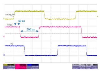
Figure 16: With external sync, the CLKOUT signal has a fixed negative pulse width of 200 ns. Delay from SYNC rising edge to CLKOUT falling edge is approximately 60 ns.
