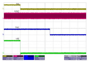
Figure 34: As long as EN = H, the IC does not shut down VDD and CLKOUT. But internal latched faults are cleared by PWM = L for  $\sim$ 16 ms.
