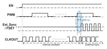
Figure 12: Avoid switching over between Internal Oscillator and External Sync in highlighted region
