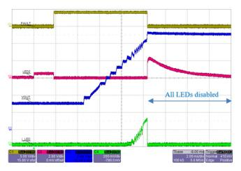
Figure 41: A80606-1 startup with LED2 string open. V<sub>OUT</sub> hits OVP and all LED string are disabled. FAULT pin goes Low and IC remains latched off until reset.
