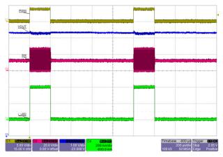
Figure 17: PWM dimming operation at 20% 1 kHz. CH1 = PWM (5 V/ div), CH2 = SW (20 V/div), CH3 =  $V_{OUT}$ , CH4 =  $i_{LED}$  (200 mA/div).
