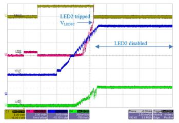
Figure 38: A80606 startup sequence when LED string#2 has a partialshort fault (6 × WLED instead of 8). As soon as LED2 pin rises above  $V_{LEDSC}$  (~5 V), the channel is disabled and FAULT = Low.
