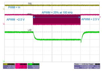
Figure 27: PWM = H. Total LED current drops from 400 mA (4 × 100 mA/ch) to 300 mA when APWM of 25% duty cycle is applied. Note that LED current takes ~1 ms to settle after change in APWM.
