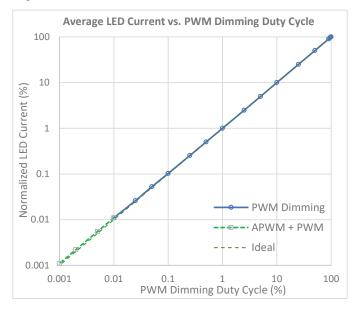
Figure 29: How to achieve 100,000:1 dimming ratio by using both PWM and APWM. Test conditions:  $V_{IN}$  = 12 V,  $V_{OUT}$  = 25 V (8 × WLED), total LED current = 400 mA, PWM frequency = 200 Hz, APWM frequency = 100 kHz.
