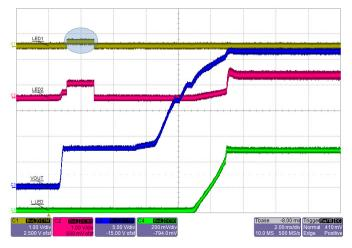
Figure 7: Normal startup showing LED1 channel is disabled with a 4.75 k $\Omega$  resistor to GND. Total LED current = 100 mA × 5.
