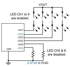
Figure 5: How to signal an unused LED channel during startup LED detection phase
