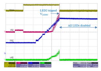
Figure 39: A80606-1 startup sequence when LED string#2 has a partial-short fault (6 × WLED instead of 8). As soon as LED2 pin rises above  $V_{LEDSD}$  (~5 V), the channel is disabled but FAULT remains High.
