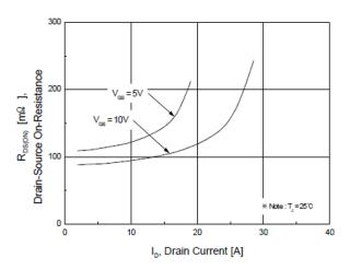
Figure 56: Chart showing On-Resistance varies with Darin Current and Gate Voltage.
