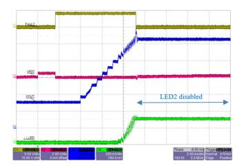
Figure 40: A80606 startup with LED2 string open. V<sub>OUT</sub> hits OVP at ~28 V and LED2 is removed from regulation. FAULT pin goes Low but remaining LED strings continue to operate.
