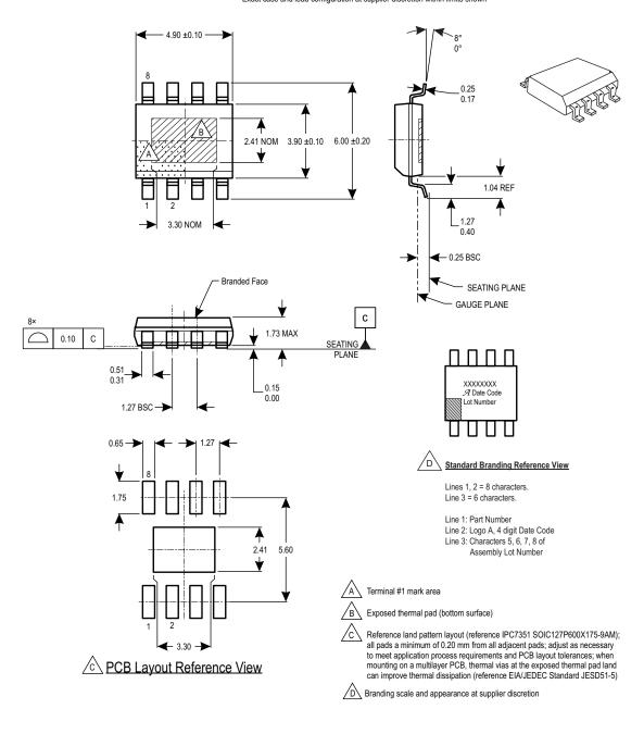
Package LJ 8-Pin SOIC with Exposed Thermal Pad
