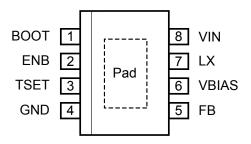
Package LJ, 8-Pin SOIC Pinout Diagram
