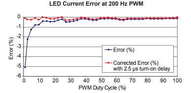
The LED Current Error graph shows the effect of PWM duty cycles on LED current error, according to the relationship:
