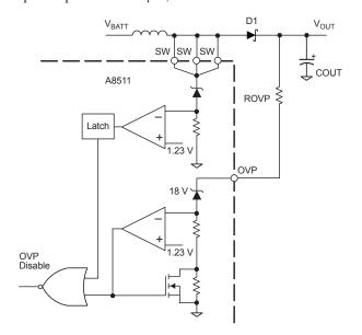
Figure 3. Overvoltage protection (OVP) circuit
