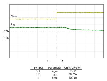
Figure 4. Output overvoltage protection (OVP) operation
