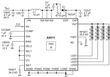
Figure 9. Typical circuit as SEPIC converter (SEPIC converters can provide output voltage higher or lower than the input voltage; this topology can be used if the required output voltage level is within application input voltage range)
