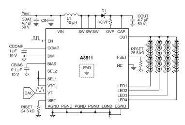
Figure 7. Typical circuit for analog dimming with external DC voltage
