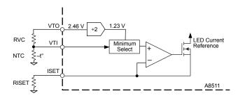
Figure 5. Thermal derating reference circuit
