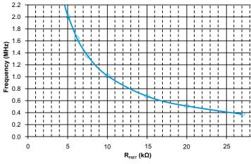
Figure 9: Boost Switching Frequency as a Function of FSET Resistance
