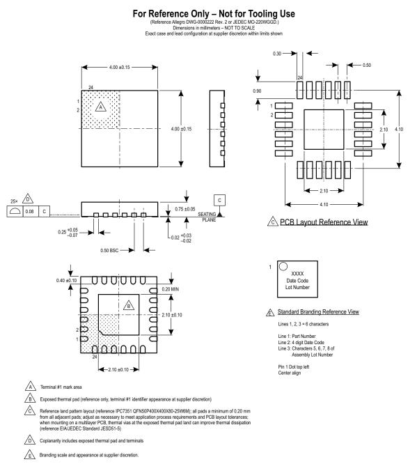
Figure 20: Package ES, 24-Pin 4 mm × 4 mm QFN with Exposed Thermal Pad
