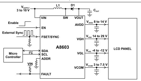
System Block Diagram Showing Typical Regulator Voltages
