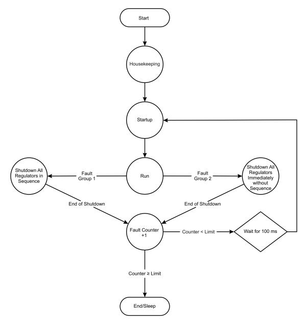
Figure 18: Fault-Retry Counter
