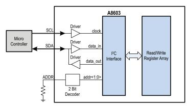
Figure 1: I<sup>2</sup>C Serial Interface and Programmable Memory Array
