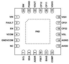
Package ES, 24-Pin QFN Pinouts
