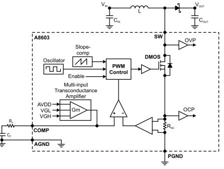
Figure 8: Boost Controller Circuit
