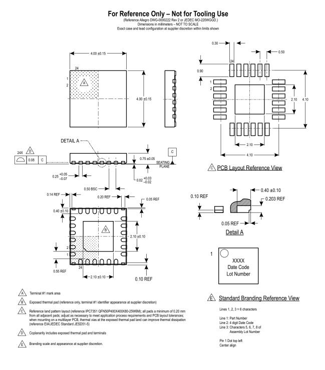
Figure 21: Package ES, 24-Pin 4 mm × 4 mm QFN with Exposed Thermal Pad and Wettable Flank
