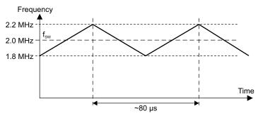
Figure 11: Switching Frequency Varied Linearly In this example, Reg0x10 = '10' and the central switching frequency is  $f_{SW} = 2.0$  MHz. The actual frequency is varied linearly between  $f_{SW} - 10\%$  and  $f_{SW} + 10\%$  by the modulating frequency at 12 kHz.
