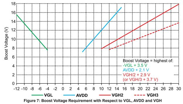
For example: assume the output requirements for a certain LCD panel are:  $V_{AVDD} = 10$  V,  $V_{VGH} = 18$  V and  $V_{VGL} = -7$  V, then:
