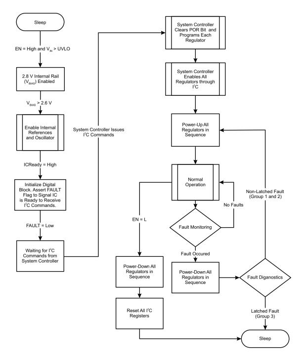
Figure 17: Fault Checking During Startup and Normal Operation
