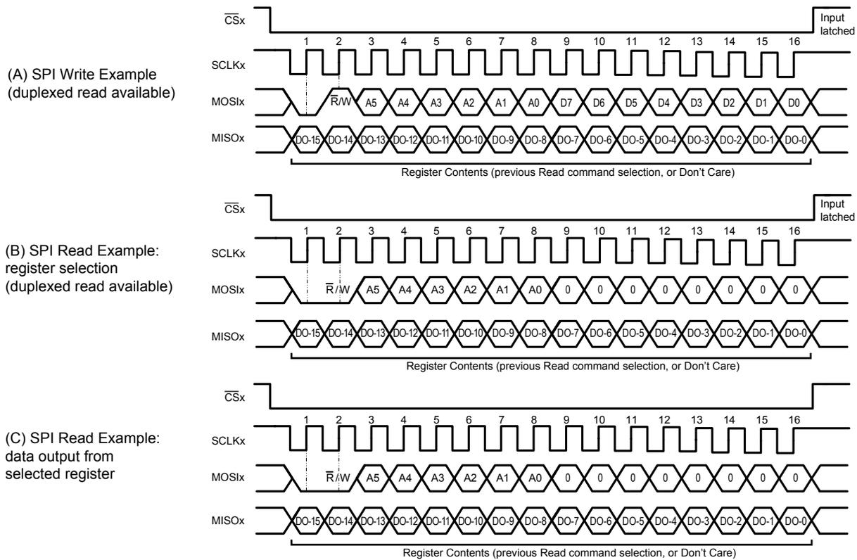
**Figure 21: SPI Read and Write Pulse Sequences**
