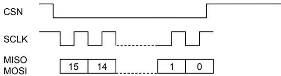
**Figure 18: 16-Bit SPI Frame**
