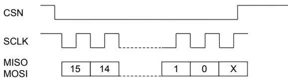
**Figure 19: 17-Bit SPI Frame**
