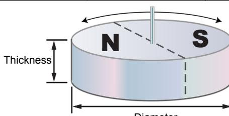
\* A sintered Neodymium magnet with 10 mm (or greater) diameter and 2.5 mm thickness is the recommended magnet for redundant applications.
