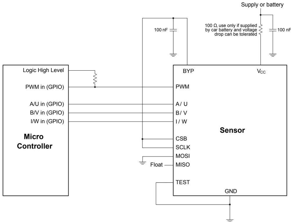
**Figure 34: Typical ABI / UVW Application Diagram**
