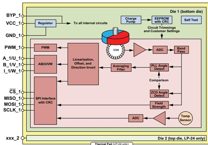
**Figure 1: AAS33001 Magnetic Circuit and IC Diagram**
