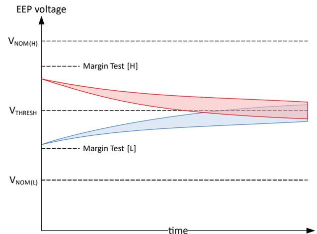
**Figure 31: Example of failing programming voltages**
