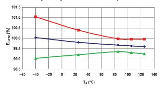
**Total Output Error versus Ambient Temperature**
