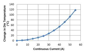
Figure 3: Self-Heating in the EX Package
