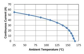
Figure 2: Maximum Continuous Current in the LC Package at a Given T<sub>A</sub>
