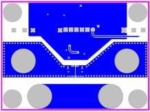
Figure 5: Top and Bottom Layers for ASEK711 Evaluation Board (TED-85-0404-001)
