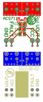
Figure 6: Top and Bottom Layers for ASEK711 Evaluation Board (TED-85-0595-001)
