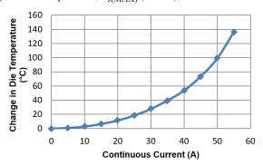
Figure 1: Self-Heating in the LC Package
