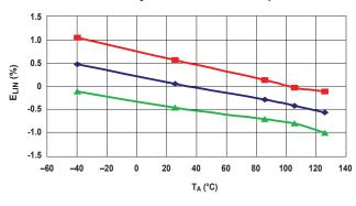
**Symmetry versus Ambient Temperature**
