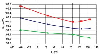
**Total Output Error versus Ambient Temperature**
