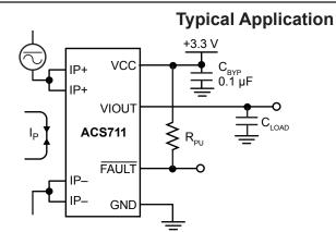
Application 1. The ACS711 outputs an analog signal,  $V_{IOUT}$ , that varies linearly with the bi-directional AC or DC primary current,  $I_P$ , within the range specified. The FAULT pin trips when  $I_P$  reaches  $\pm 100\%$  of its full-scale current.
