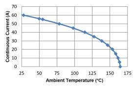
Figure 4: Maximum Continuous Current in the EX Package at a Given T<sub>A</sub>
