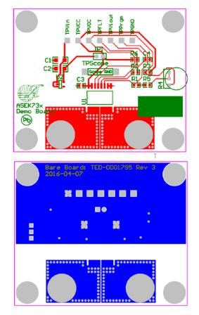
Figure 10: Top and Bottom Layers for ASEK73x Evaluation Board
