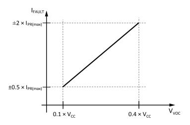
Figure 4: Fault Threshold vs. V<sub>VOC</sub>
