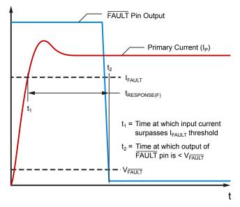
Figure 3: Overcurrent Fault Response
