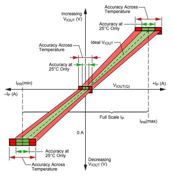
Figure 5: Output Voltage versus Sensed Current
