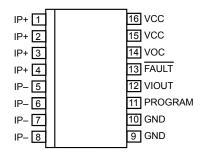
Package LA, 16-Pin SOICW Pinout Diagram
