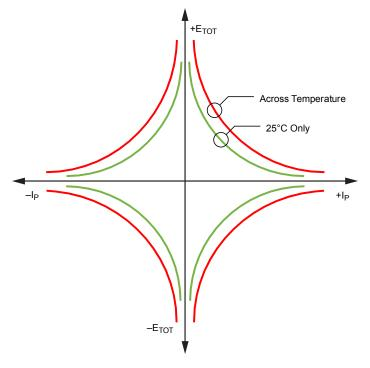
Figure 6: Total Output Error versus Sensed Current
