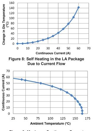
Figure 9: Maximum Continuous Current at a Given T<sub>A</sub>
