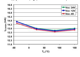
**Supply Current Ratio versus Ambient Temperature**
