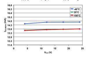
Supply Current (High) versus Ambient Temperature
