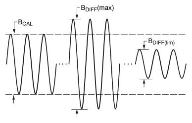
Figure 11. Illustration of  $B_{CAL}$ ,  $B_{DIFF}(max)$  and  $B_{DIFF(lim)}$  for amplitude variation discussion.  $B_{CAL}$  is the magnetic amplitude at the IC during its calibration cycle  $B_{DIFF}(max)$  and  $B_{DIFF(lim)}$  are the maximum and minimum magnetic amplitudes during IC operation.
