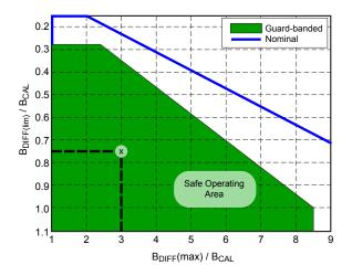
Figure 10. Allowable Signal Amplitude Change chart
