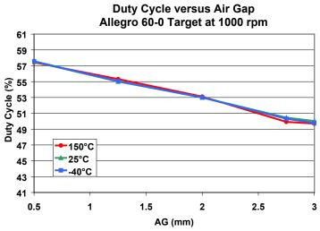
The trend of duty cycle versus air gap is driven by the actual magnetic profile of the target (see Reference Target figures)
