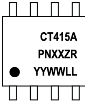
Figure 22: CT415 Device Marking for 8-lead Package
