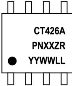
Figure 44: CT426 Device Marking for 8-lead Package
