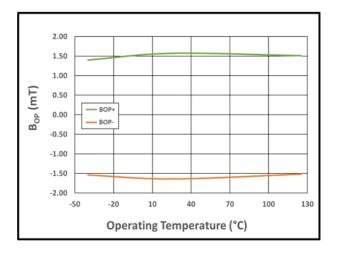
Figure 23:  $B_{OP-}$  (Orange) and  $B_{OP+}$  (Green) vs. Temperature at  $V_{DD}$  = 3.3 V
