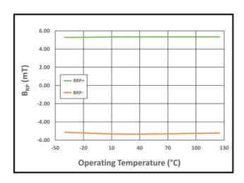
Figure 31:  $B_{RP-}$  (Orange) and  $B_{RP+}$  (Green) vs. Temperature at  $V_{DD}$  = 3.3 V
