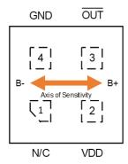
Figure 5: CT8132 4-Lead LGA Package with Digital Output (Top View)
