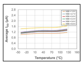
Figure 19: Average Supply Current vs. Temperature vs. Supply Voltage
