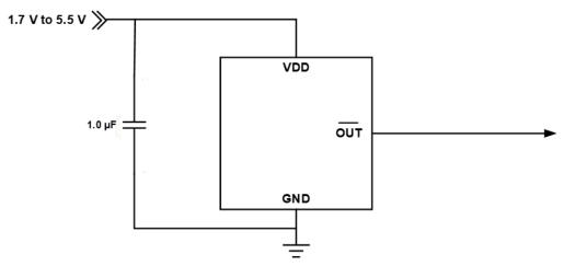
Figure 48: CT8132 Application Block Diagram
