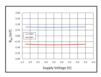
Figure 22:  $B_{RP-}$  (Red) and  $B_{RP+}$  (Blue) vs. Supply Voltage at  $T_A = 25$ °C
