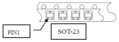
Figure 54: SOT23 Orientation in Tape Pocket
