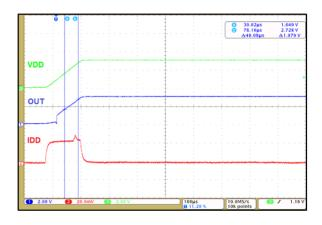
Figure 6: Power-On Time for Push-Pull Output
