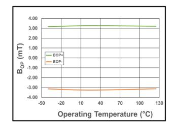
Figure 10:  $B_{OP-}$  (Orange) and  $B_{OP+}$  (Green) vs. Temperature at  $V_{DD}$  = 3.3 V
