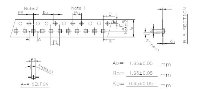
Figure 55: Tape and Pocket Drawing for LGA-4 Package
