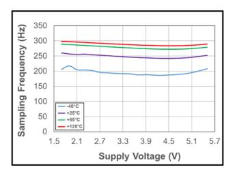
Figure 44: Sampling Frequency vs. Supply Voltage vs. Temperature
