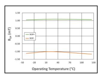
Figure 38:  $B_{RP-}$  (Orange) and  $B_{RP+}$  (Green) vs. Temperature at  $V_{DD}$  = 3.3 V
