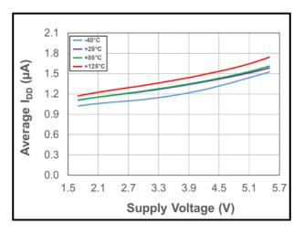
Figure 18: Average Supply Current vs. Supply Voltage vs. Temperature
