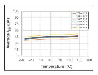
Figure 16: Average Supply Current vs. Temperature vs. Supply Voltage
