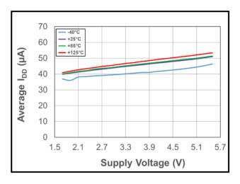
Figure 15: Average Supply Current vs. Supply Voltage vs. Temperature
