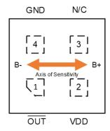
Figure 4: CT8131 4-Lead LGA Package with Digital Output (Top View)
