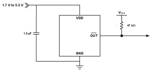
Figure 47: CT8131 Application Block Diagram
