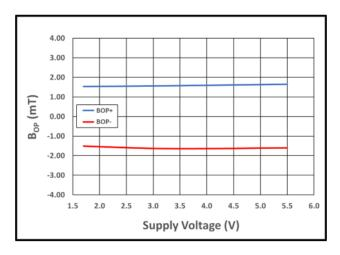
Figure 21:  $B_{OP-}$  (Red) and  $B_{OP+}$  (Blue) vs. Supply Voltage at  $T_{\Delta}$  = 25°C
