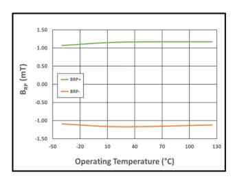
Figure 24:  $B_{RP-}$  (Orange) and  $B_{RP+}$  (Green) vs. Temperature at  $V_{DD}$  = 3.3 V
