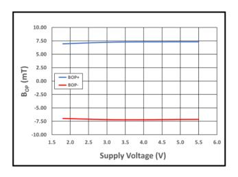
Figure 28:  $B_{OP-}$  (Red) and  $B_{OP+}$  (Blue) vs. Supply Voltage at  $T_A = 25$ °C
