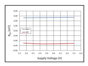
Figure 29:  $B_{RP-}$  (Red) and  $B_{RP+}$  (Blue) vs. Supply Voltage at  $T_A = 25$ °C
