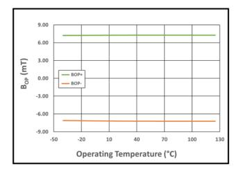
Figure 30:  $B_{OP-}$  (Orange) and  $B_{OP+}$  (Green) vs. Temperature at  $V_{DD}$  = 3.3 V
