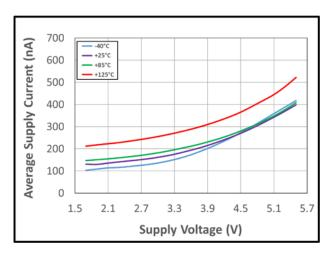
Figure 32: Average Supply Current vs. Supply Voltage vs. Temperature
