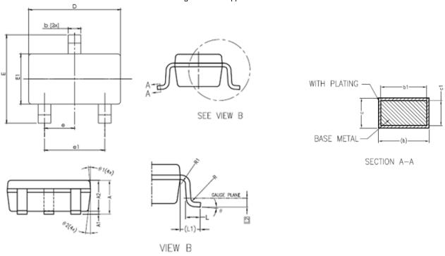
Figure 51: 3-Lead SOT23 Package Drawing
