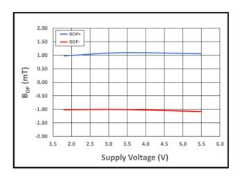
Figure 35:  $B_{OP-}$  (Red) and  $B_{OP+}$  (Blue) vs. Supply Voltage at  $T_A = 25$ °C
