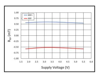
Figure 36:  $B_{RP-}$  (Red) and  $B_{RP+}$  (Blue) vs. Supply Voltage at  $T_A = 25$ °C
