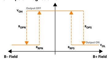
Figure 46: CT813x Response Time Curve
