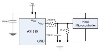
Figure 3: A31315 Typical Application Circuit (Analog Interface)
