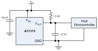
Figure 2: A31315 Typical Application Circuit (Digital Interface)
