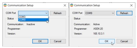
6. Setup the device communication: Under the Setup tool bar, click "Device Setup...". This opens a new pop-up window.
