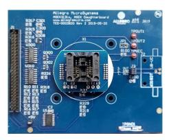
B. Insert an A31315 device into the socket. The A31315 device should be placed such that the pin identifier (denoting pin 1) is at the top left.
