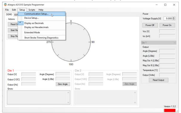
5. Select the COM port associated with the ASEK-20 device. Once the correct COM port is selected, the Status info box populates with information about the ASEK firmware. If an incorrect COM port is selected, the GUI attempts to communicate with the port until it ultimately times out.
