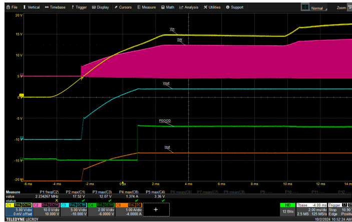
Figure 3: Startup, 8.6 Ω Load, Enable = VIN, VIN = 18 V
