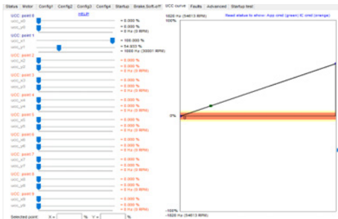
Figure 43: UCC Set to Maximum Speed For Motor Used
