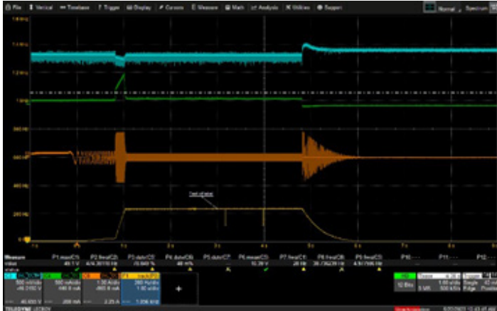
Figure 37: Pulsed Low-Side Braking
