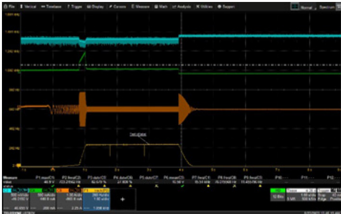
Figure 38: Continuous Low-Side Braking
