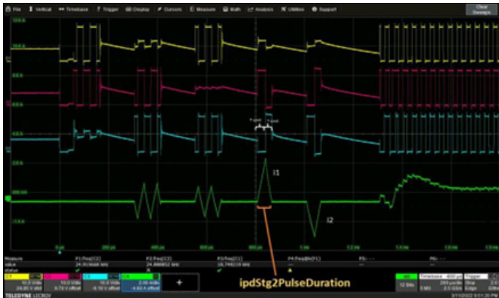
Figure 35: Output Voltages and Phase A Current
