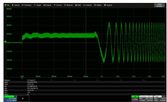
Figure 21: K_i Instabilities—GUI Plot (left) and Phase Current Plot (right)
