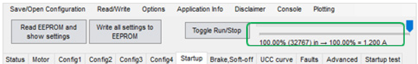
Figure 16: Command Slider, Showing 100% Demand Equal To Maximum System Current
