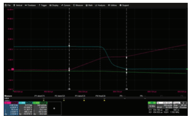
Figure 11: Turn-Off and Turn-On Behavior—C2 Power MOSFET, V_{GS} ; C3 Power MOSFET, V_{DS}
