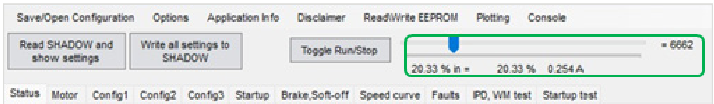
Figure 15: Command Slider in Torque Mode, Showing Current as Reference
