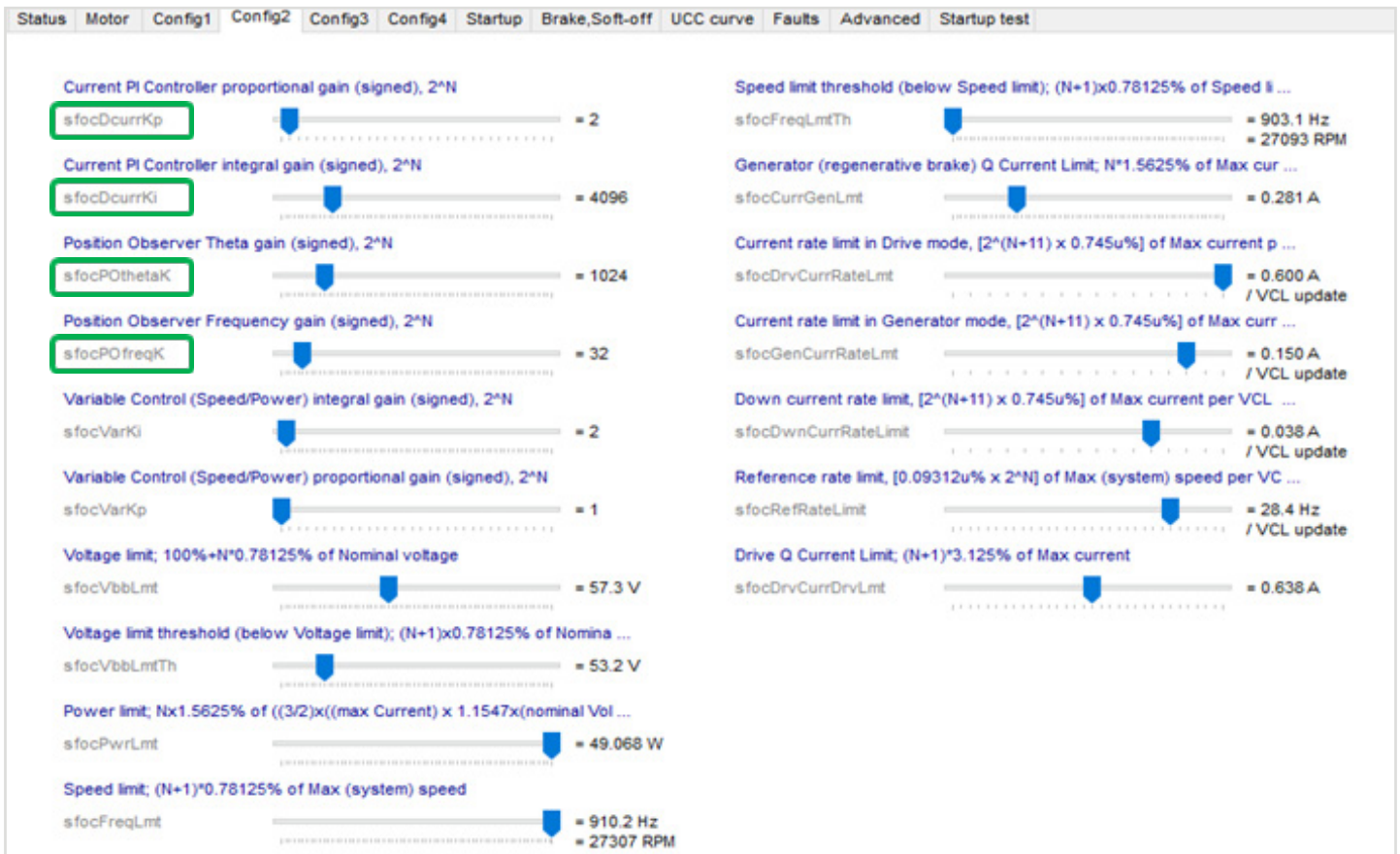
Figure 23: Closed-Loop Current PI and Observer Parameters
