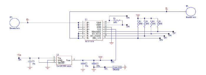
Figure 2: Schematic for ACS71020 Evaluation Board
