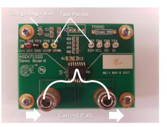
Figure 1: Allegro ACS71020 Current Sensor Evaluation Board
