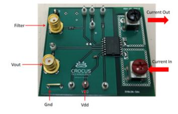
Figure 1: CT431-20AC Evaluation Board
