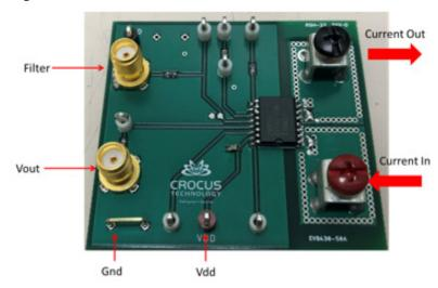
Figure 2: CT431-20AC Evaluation Board
