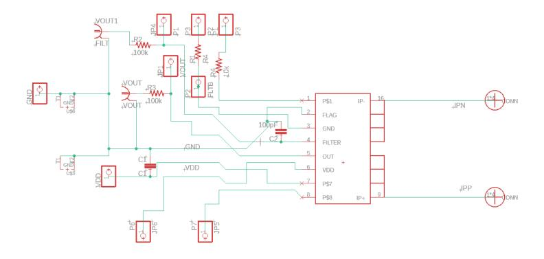
Figure 4: CT431-20AC Evaluation Board Schematic
