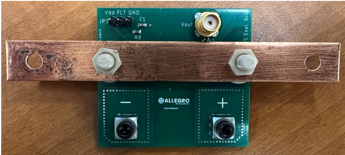
Figure 2: CTD455-BB-06B5 Evaluation Board with Busbar
