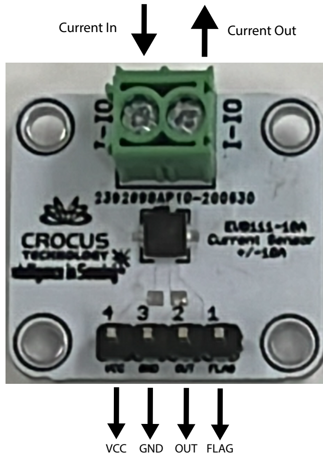
Figure 2: EVB111-10A evaluation board connections
