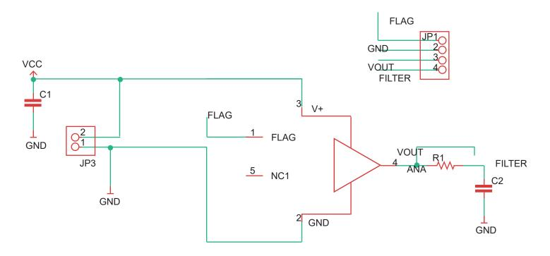
Figure 3: EVB222-1.5 Evaluation Board Schematic
