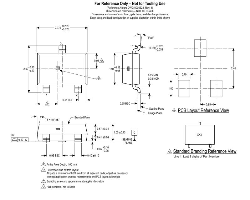
Figure 9: Package LH, 3-Pin SOT23W (A1130LLH, A1131ELH, A1132KLH)
