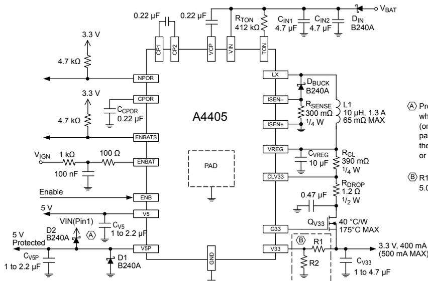
(A) Protection diodes D1 and D2 are required when the V5P pin is driving a wiring harness (or excessively long PCB trace) where parasitic inductance will cause the voltage at the V5P to momentarily transition above VIN or below ground during a fault condition.
