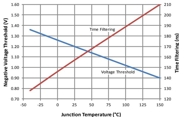
Figure 2. Missing diode protection versus device junction temperature
