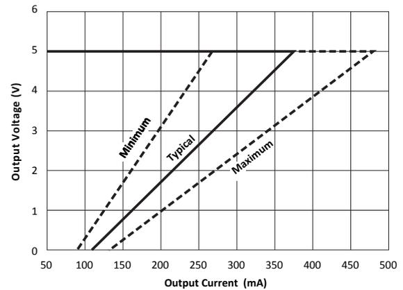
Figure 5. Foldback current limit of the 5VP regulator
