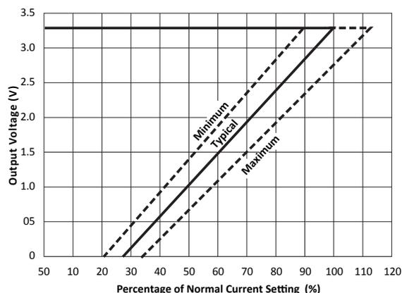
Figure 8. Foldback current limit of the V33 regulator
