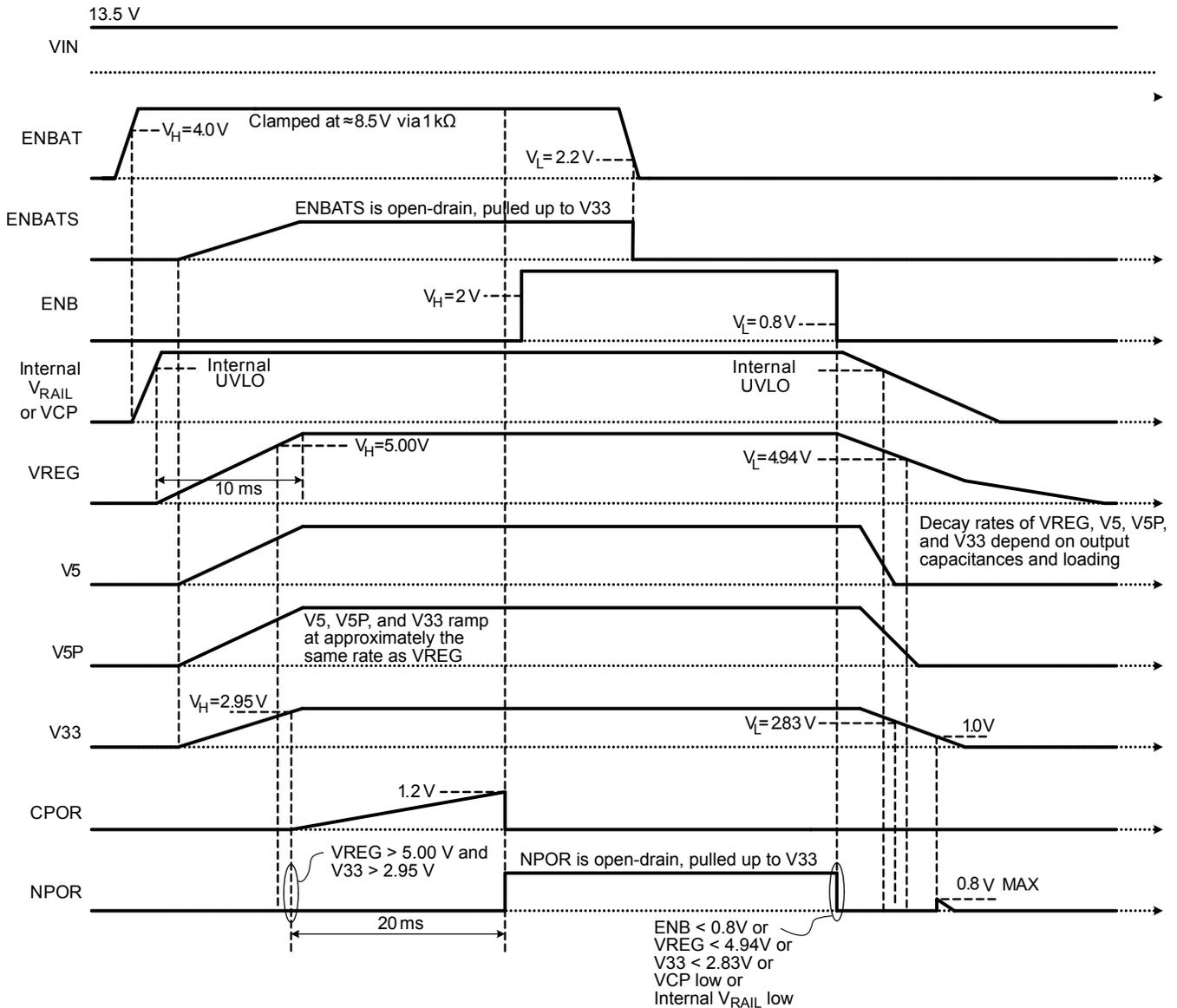
Typical power-up and power-down by ENBAT and ENB with  $V_{IN} = 13.5\text{V}$ ; ENBATS is assumed to be connected to V33 via a pull-up resistor
