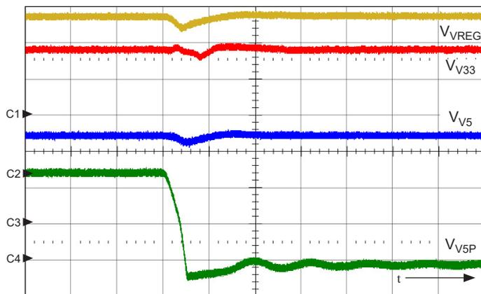
Figure 6. V5P is shorted to ground in 5  $\mu$ s ( $D_{V5P}$  is populated); shows  $V_{VREG}$  (ch1, 2 V/div.),  $V_{V33}$  (ch2, 1 V/div.),  $V_{V5}$  (ch3, 2 V/div.),  $V_{V5P}$  (ch4, 2 V/div.),  $t = 10 \mu$ s/div.
