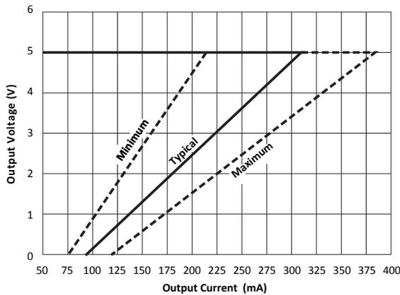
Figure 4. Foldback current limit of the 5V regulator
