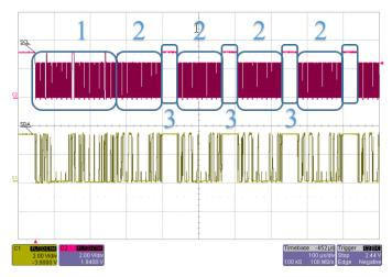
Figure 10: I<sup>2</sup>C read of 8 data bytes in Full Loop Mode. Registers 0x28 and 0x29.
