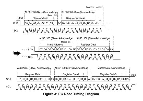
The timing diagram in Figure 4 shows the entire contents (bits 31:0) of a single register location being transmitted. Optionally, the I<sup>2</sup>C Master may choose to replace the NACK with an ACK instead, which allows the read sequence to continue. This case will result in the transfer of contents (bits 31:24) from the following register, address + 1. The master can then continue acknowledging, or issue the not-acknowledge (NACK) or stop after any byte to stop receiving data.
