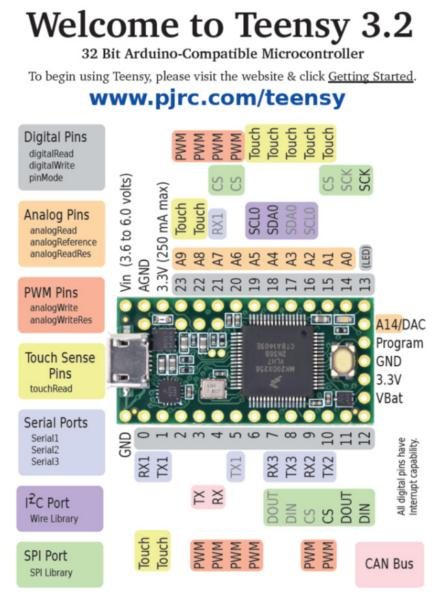
Figure 13: Pinout Flyer for TEENSY 3.2
