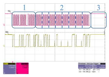
Figure 9: I<sup>2</sup>C read of 8 data bytes in No loop mode. Registers 0x28 and 0x29.
