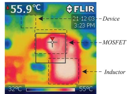
Figure 12: Thermal performance with  $I_{LED} = 400$  mA at 12 V input and room temp for low-beam operation (7 LEDs).
