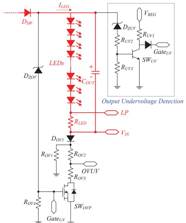
Figure 17: Additional circuit for the output undervoltage protection.
