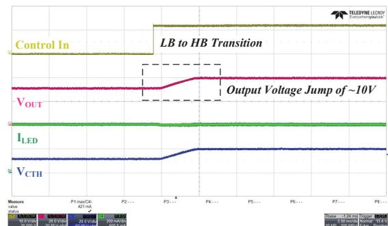
Figure 14: Transient behavior during low-beam to high-beam transition.
