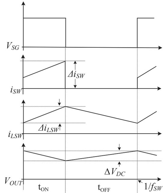
Figure 3: Waveforms of the operation of buck-boost converter in CCM.
