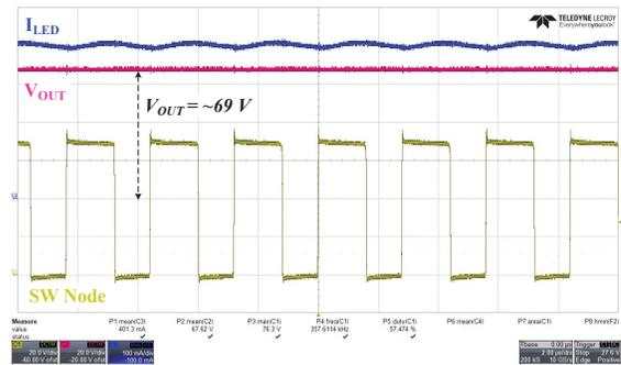
Figure 6: Steady-state operating waveforms for 10 LEDs (high-beam) for an input voltage of 40 V.
