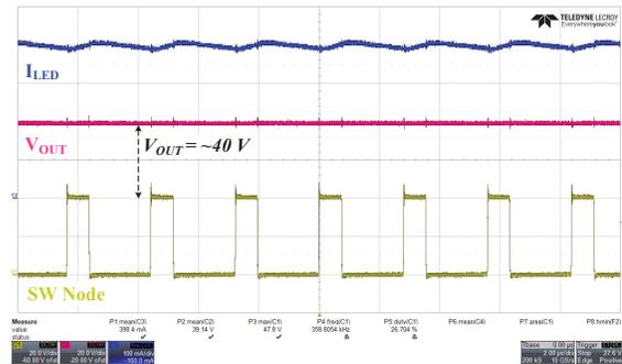
Figure 5: Steady-state operating waveforms for 10 LEDs (high-beam) for an input voltage of 12 V.
