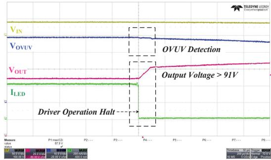
Figure 15: Overvoltage detection during open-LED operation.
