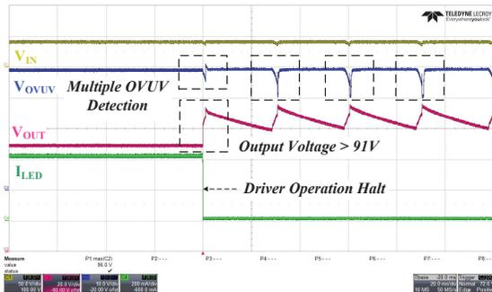
Figure 16: Hiccup operation during the overvoltage protection.
