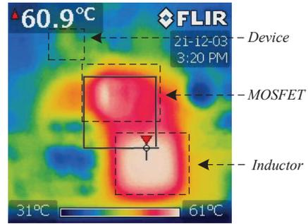
Figure 11: Thermal performance with  $I_{LED} = 400$  mA at 12 V input and room temp for high-beam operation (10 LEDs).
