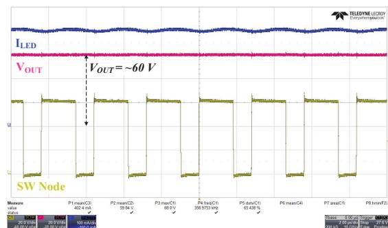
Figure 8: Steady-state operating waveforms for 7 LEDs (low-beam) for an input voltage of 40 V.
