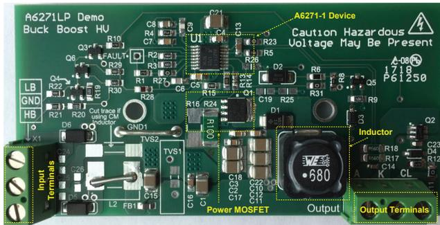
Figure 4: High-voltage experimental board using A6271-1.
