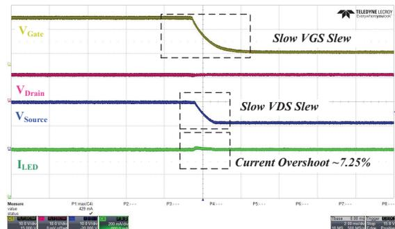
Figure 20: High-beam to low-beam transition with added gate-drain capacitance of 100 nF to the bypass MOSFET.
