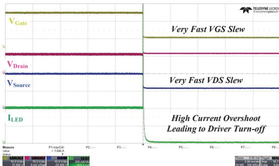
Figure 18: High-beam to low-beam transition with no added capacitance to the bypass MOSFET.
