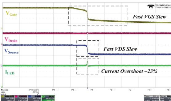
Figure 19: High-beam to low-beam transition with added gate-source capacitance of 1  $\mu\text{F}$  to the bypass MOSFET.
