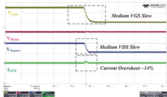
Figure 21: High-beam to low-beam transition with added gate-drain capacitance of 47 nF to the bypass MOSFET.
