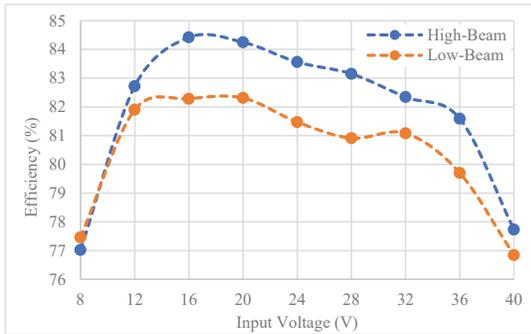
Figure 9: Plot of efficiency vs. input voltage for high-beam and low-beam operation of buck-boost converter using A6271-1.
