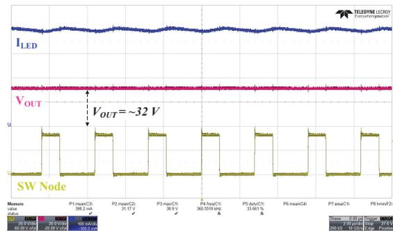
Figure 7: Steady-state operating waveforms for 7 LEDs (low-beam) for an input voltage of 12 V.
