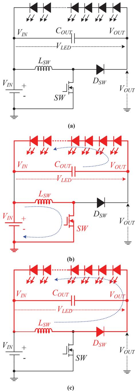
Figure 2: Buck-boost converter (a) Simplified power stage, (b) Operation during the switch-on period, (c) Operation during the switch-off period.
