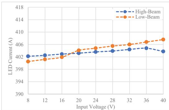
Figure 10: Plot of regulated LED current vs. input voltage for high-beam and low-beam operation of buck-boost converter using A6271-1.
