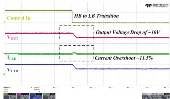
Figure 13: Transient behavior during high-beam to low-beam transition.
