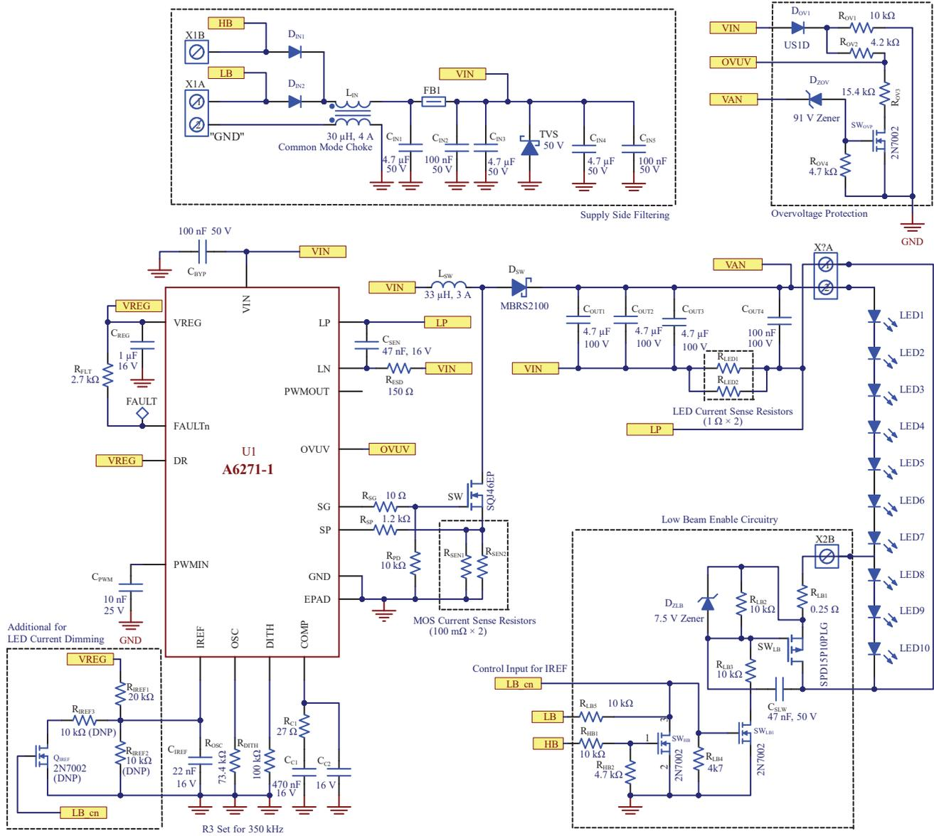
Figure 22: Schematic of the automotive headlamp application.
