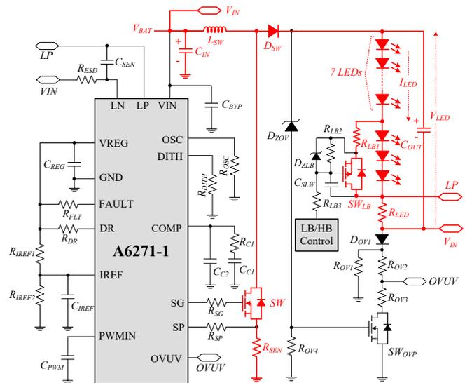
Figure 1: High-voltage buck-boost configuration using A6271-1.
