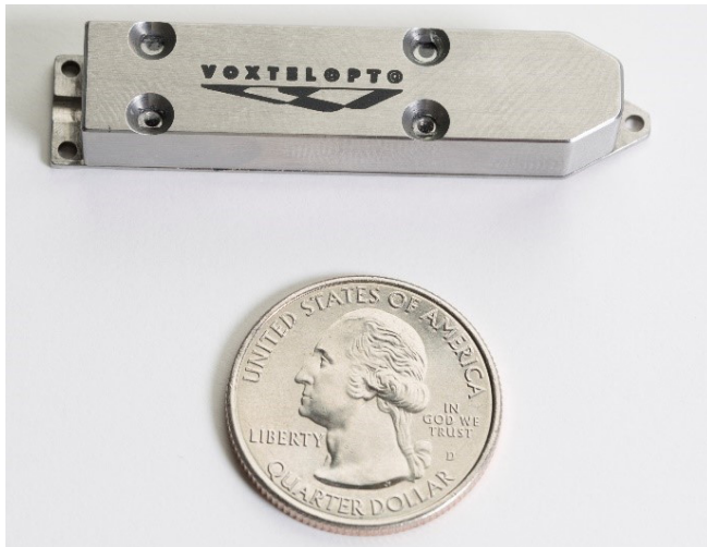
Figure 5: The Allegro test laser—a miniature 1535 nm DPSS laser, shown in comparison to the size of a quarter—has a beam quality of M^2 < 1.1 \times DL (diffraction limit) and can be operated at 20 \mu J at up to a 400 kHz repetition rate. The laser was developed by the Allegro photonics group, then operating as Voxel.
