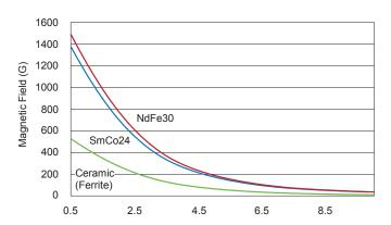
**Figure 31:** Magnetic Field versus Air Gap for a magnet 6 mm in diameter and 2.5 mm thick. Allegro can provide similar curves for customer application magnets upon request. Allegro recommends larger magnets for applications that require optimized accuracy performance.
