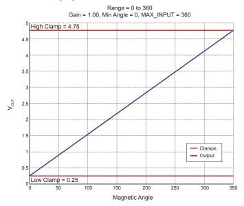
**Figure 25: Scenario A.**Regular output for a 0-360 degree input angle.
