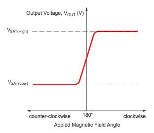
Figure 41: Effect of Saturation
