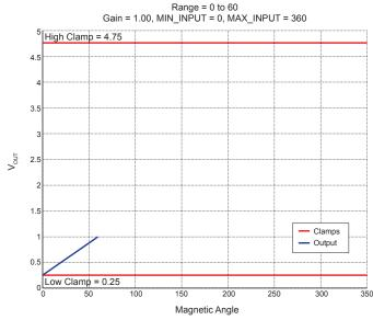
**Figure 27: Scenario C.**0-60 degree input. Gain = 1.
