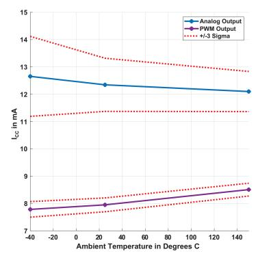
Figure 4:  $I_{CC}$  over Temperature  $(V_{CC} = 5.0 \text{ V})$
