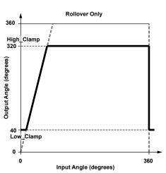
Figure 22: CE = 1, ROE = 0. Applied gain = 4×. LOW\_CLAMP = 10 (≈40°), HIGH\_CLAMP = 10 (≈320°)
