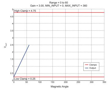
**Figure 28: Scenario D.** 0-60 degree input. Gain = 3. With an increased Gain value of 3×, the same 60-degree input signal now results in 50% of  $V_{CC}$ . The output signal is still free to swing from 5% to 95% of  $V_{CC}$ .
