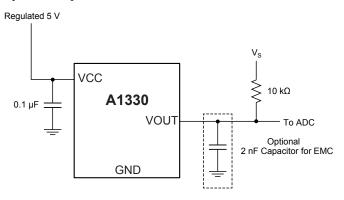
Figure 36: Typical A1330 application circuit
