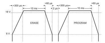
Figure 10: Top-Level Programming Interface
