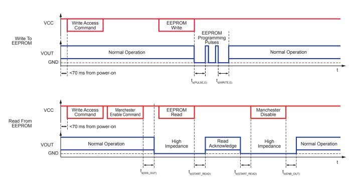
Figure 12: Programming Read and Write Timing Diagrams
