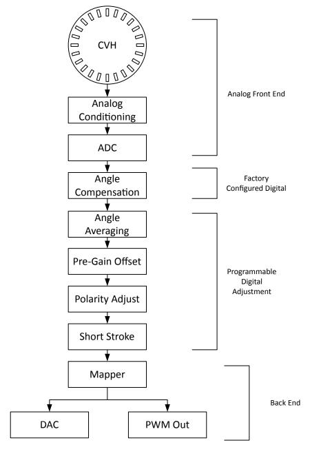
Figure 16: Digital Signal Path Description
