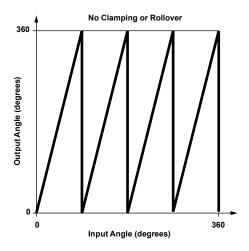
Figure 21: CE = 0, ROE = 0. Applied gain =  $4\times$ .
