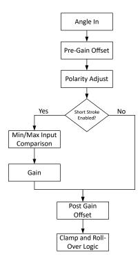
Figure 18: High Level Short Stroke Block Diagram
