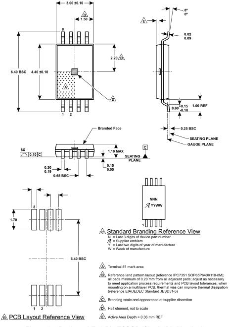
Figure 37: Package LE, 8-Pin TSSOP (Single Die Version)
