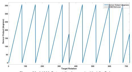
Figure 20: A1330 Output (in degrees) with 4.5× Gain
