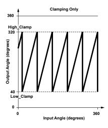
Figure 23: CE = 0, ROE = 1. Applied gain =  $4\times$ . LOW\_CLAMP = 10 ( $\approx$ 40°), HIGH\_CLAMP = 10 ( $\approx$ 320°)
