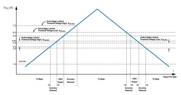
Figure 8: Relationship of V<sub>CC</sub> and Output
