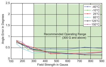
Figure 33: Typical Angle Error
