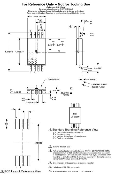
Figure 38: Package LE, 8-Pin TSSOP (Dual Die Version)
