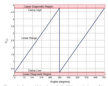
Figure 5: Output Value for a 0-720° Magnetic Input Signal
