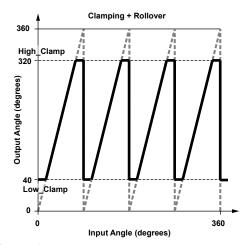
Figure 24: CE = 1, ROE = 1. Applied gain = 4×. LOW\_CLAMP = 10 (≈40°), HIGH\_CLAMP = 10 (≈320°)
