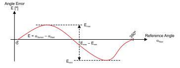
Figure 39: Angle Error Definition
