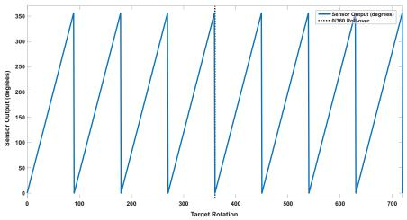
Figure 19: A1330 Output (in degrees) with 4.0× Gain
