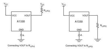
Figure 15: Connection for Detecting Broken Ground Wire
