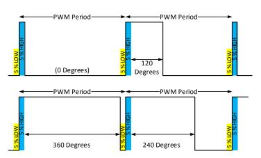
Figure 7: Pulse-Width Modulation (PWM) Examples
