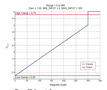
Figure 26: Scenario B. Regular 0-360 degree input value. Gain = 1. MAX\_INPUT = 300. Clamps set to 95% and 5%. Output goes into diagnostic region (in this case  $V_{CC}$ ) when input angle exceeds the MAX\_INPUT set point.
