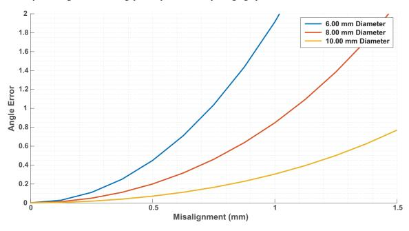
Figure 35: Simulated Error versus Eccentricity for different size magnet diameters, at 2.0 mm air gap
